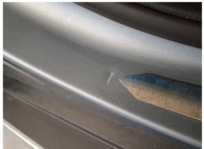
Damage 4: Sill - right side: Sill - Dent / paintcoat damage - Smart repair
