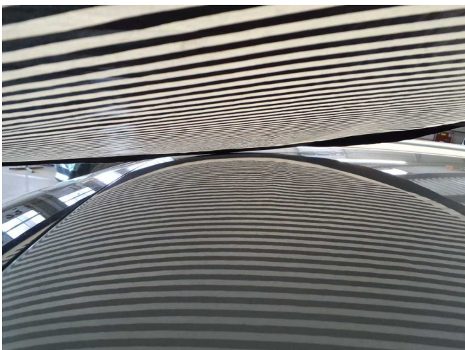
Damage 6: Roof: Roof - dent(s) - Smooth repair work
