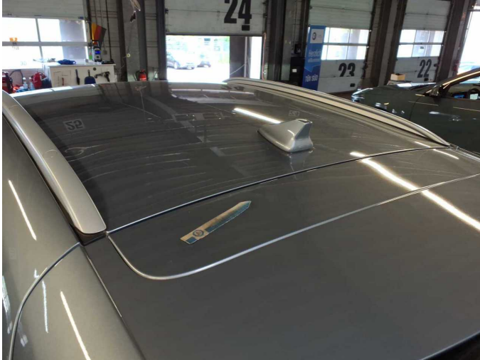
Damage 6: Roof: Roof - dent(s) - Smooth repair work
