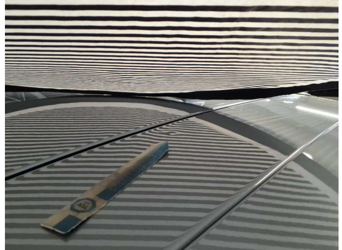
Damage 6: Roof: Roof - dent(s) - Smooth repair work
