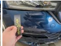
Bumper grille FR, Broken, Replace
