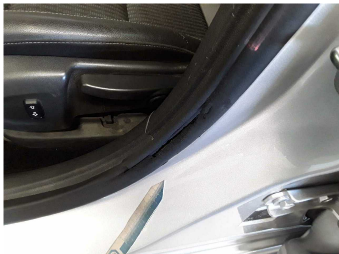
Damage 2: Cab: Door rubber seal - left side - Damaged - Replace
