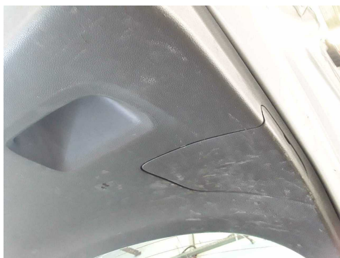
Damage 4: Trim / covers: Boot lid - interior trim - Scratched - Replace
