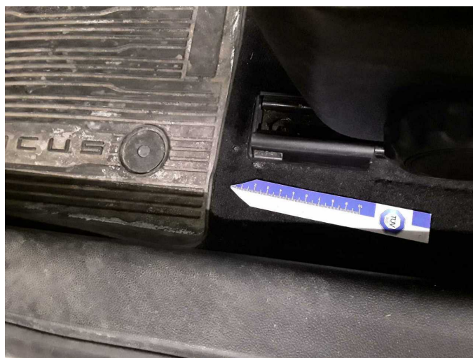
Damage 6: Trim / covers: Carpet - front left side (mehrere Brandlöcher) - Burn hole (cigarettes) - Smart repair
