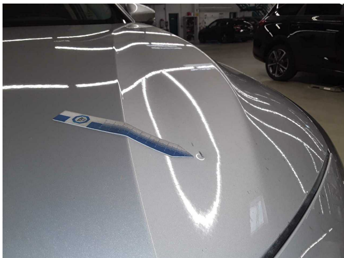
Damage 9: Bonnet: Bonnet - Dent / paintcoat damage - Paint
