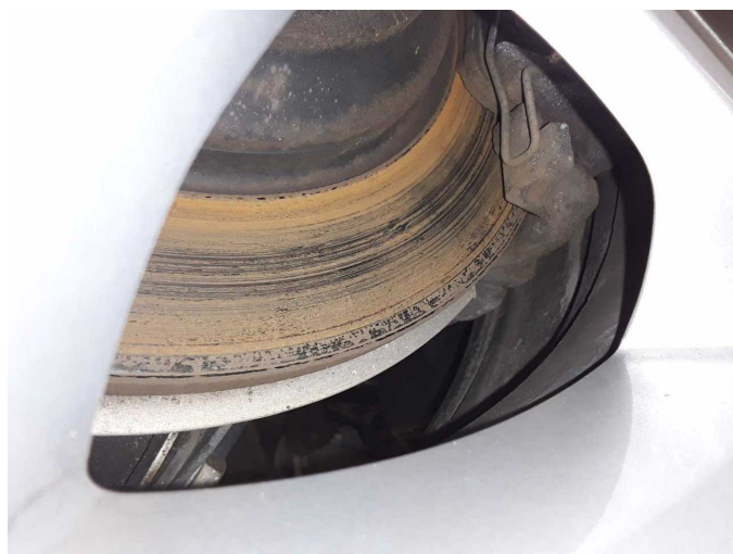
Damage 8: Braking system: Brake discs and pads - rear - Corrosion - Replace
