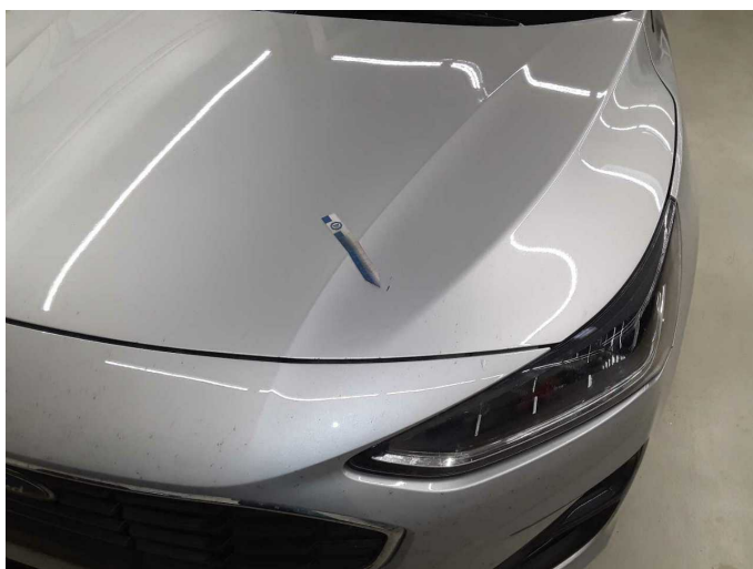
Damage 9: Bonnet: Bonnet - Dent / paintcoat damage - Paint
