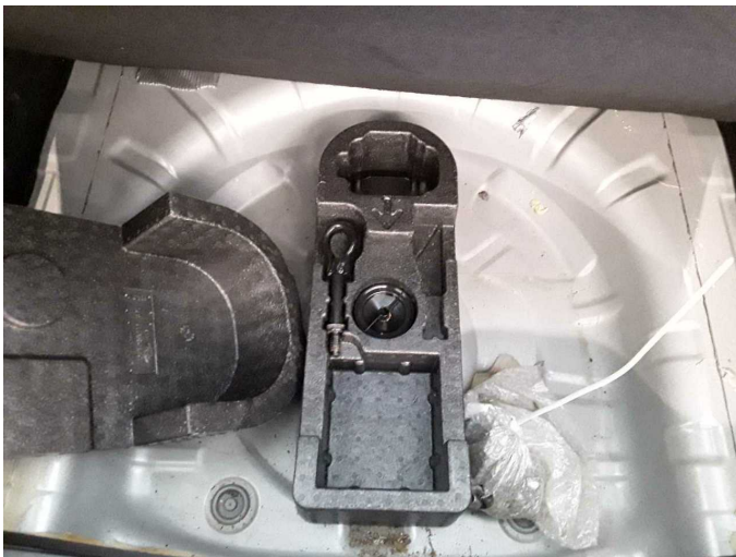
Missing part 1: Equipment: Tirefit complete - Missing - Replace
