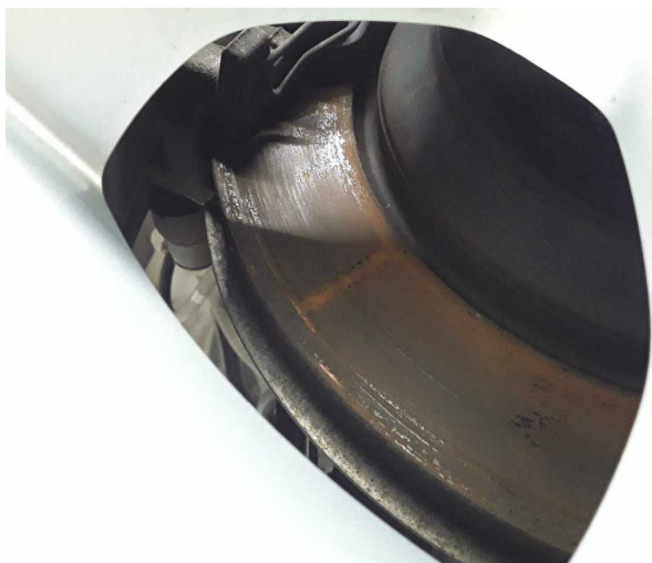
Damage 8: Braking system: Brake discs and pads - rear - Corrosion - Replace
