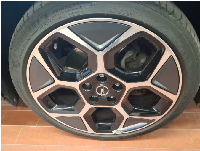
Damage 8: Wheel / tyres: Alloy rim - front right side (Optischer Mangel) - Scratched - Loss in value
