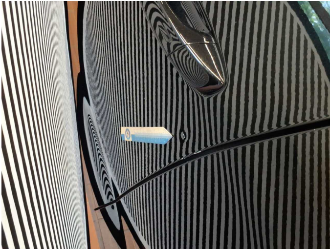
Damage 14: Door - front left side: Door - Dent / paintcoat damage - Repair and paint
