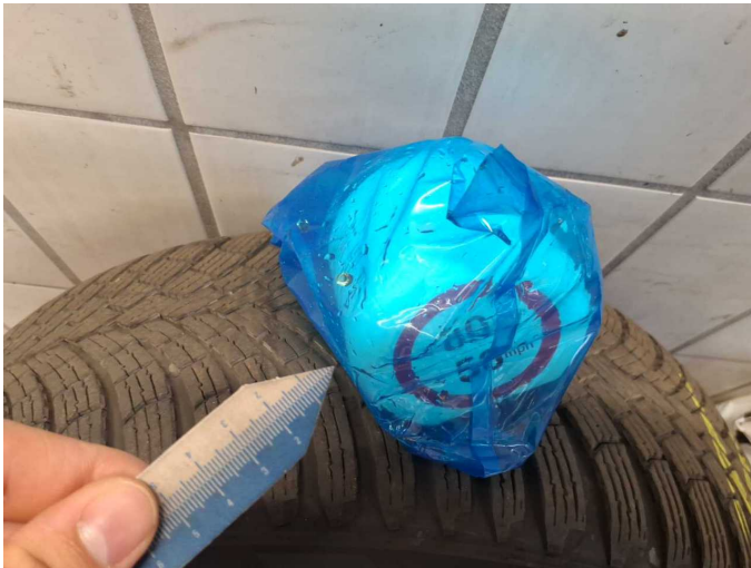
Damage 3: Equipment: Tirefit filler (Undicht) - Damaged - Replace
