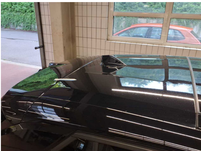
Damage 5: Roof: Roof - dent(s) - Smooth repair work
