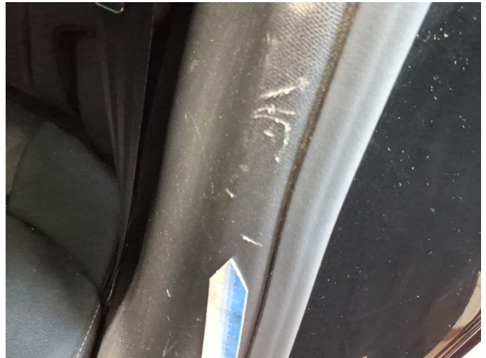
Damage 11: Trim / covers: C-pillar - trim - interior, left sde (Beschädigung zu tief) - Scratched - Replace
