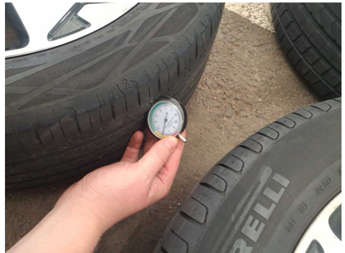
Damage 2: 2nd wheel set: 1 tyre - Does not meet the leasing specifications - Replace
