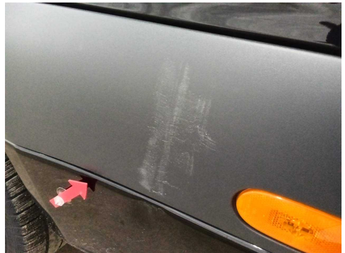
Damage 3: Side panel - rear left side: Brightware - Scratched - Replace
