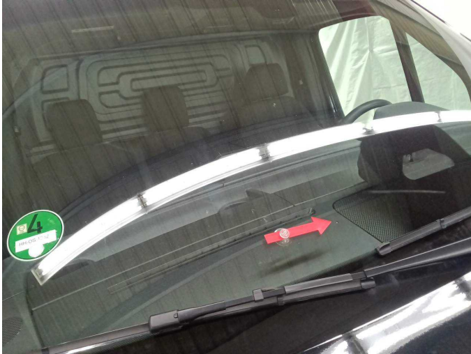
Damage 8: Vehicle glazing: Windscreen - Stone chips - Replace
