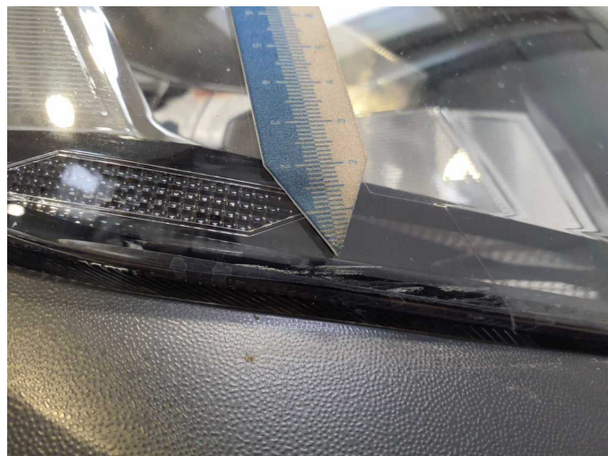
Damage 4: Headlight: Headlight - right side - Scratch(es) - Replace
