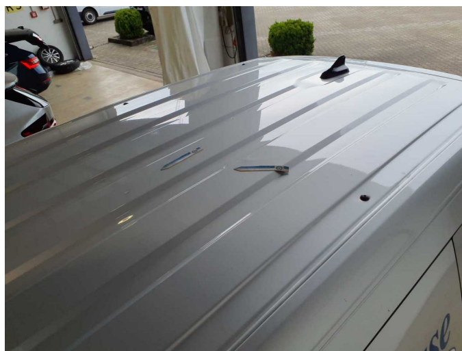
Damage 8: Roof: Roof - Deformed - Repair and paint
