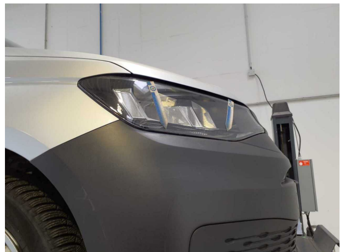
Damage 4: Headlight: Headlight - right side - Scratch(es) - Replace
