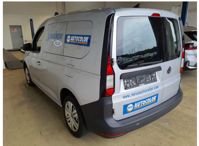
Damage 3: Body: Body - Glued / labelled - De-glue / neutralise
