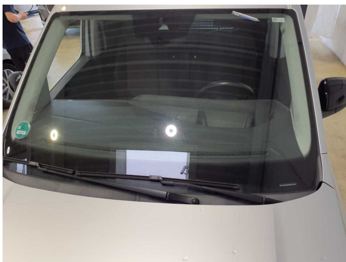
Damage 7: Vehicle glazing: Windscreen - Stone chips - Replace
