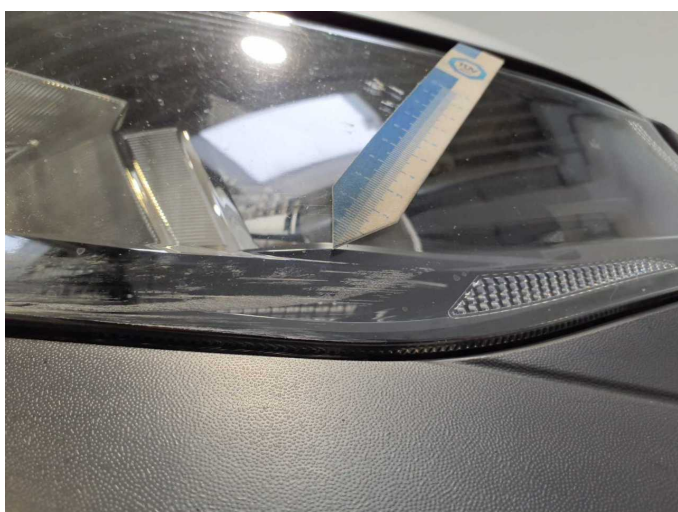
Damage 4: Headlight: Headlight - right side - Scratch(es) - Replace
