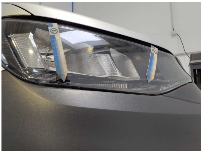
Damage 4: Headlight: Headlight - right side - Scratch(es) - Replace
