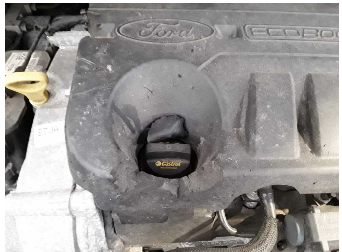
Damage 2: Engine: Engine cover - top / cover - Damage caused by marten / rodent - Replace
