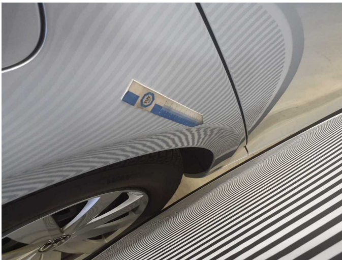
Damage 10: Side panel - rear right side: Side panel (Wellig und einschüsse) - Unprofessionally repaired - Repair and paint
