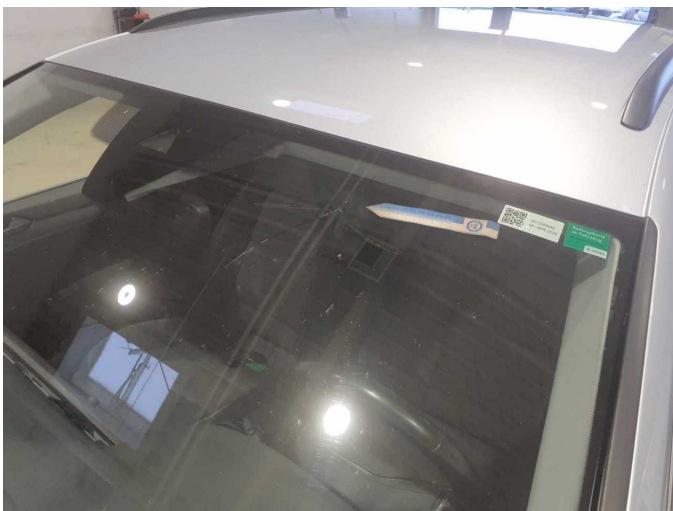
Damage 11: Vehicle glazing: Windscreen - Stone chips - repair according to calculation
