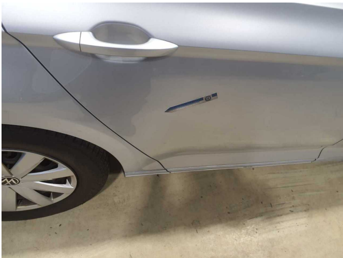
Damage 7: Door - rear right side: Door (Einschlüsse-Mehrkosten möglich) - Unprofessionally repaired - Conditioning
