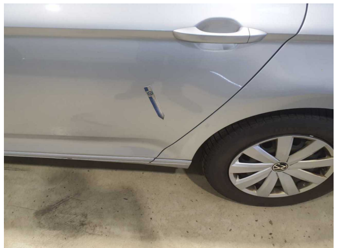
Damage 6: Door - rear left side: Door - Dent / paintcoat damage - Smart repair
