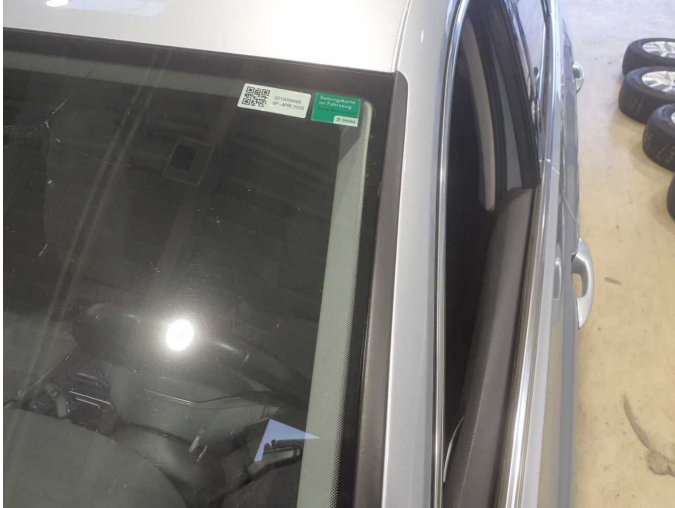
Damage 1: Trim / covers: A-pillar - trim - interior, left side - Loose - Repair
