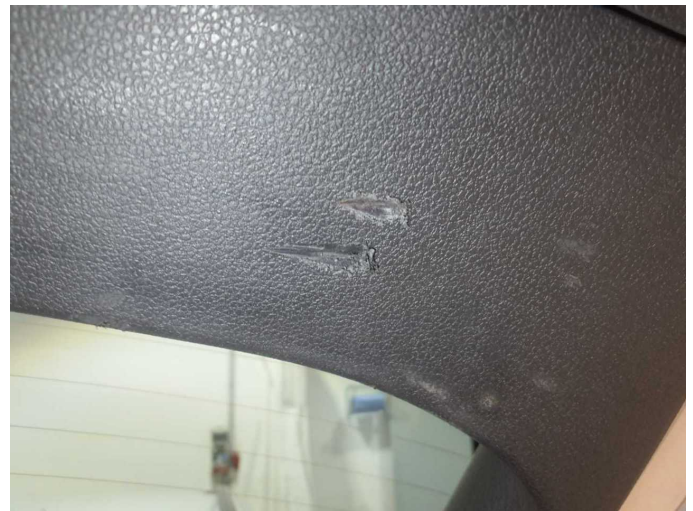
Damage 2: Trim / covers: Boot lid - interior trim - Scratch(es) - Smart repair
