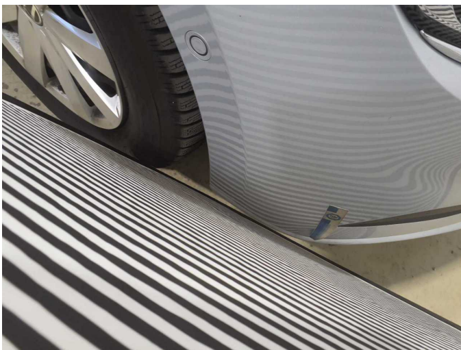
Damage 8: Front bumper: Spoiler - Broken / torn - Replace
