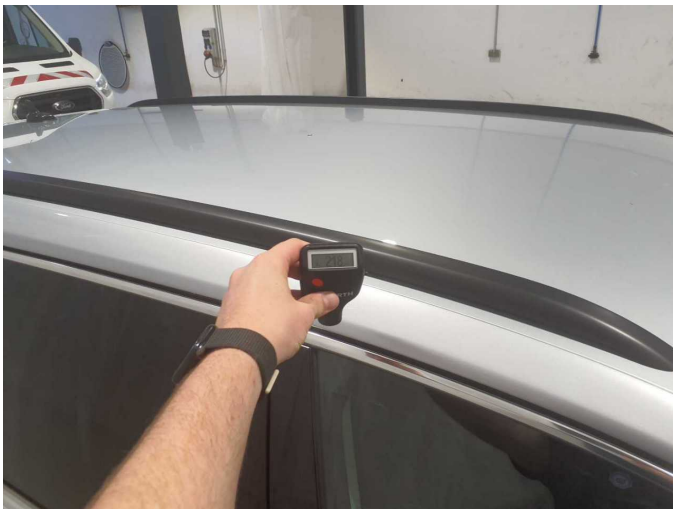
Repainting 1: Roof rail - right side
