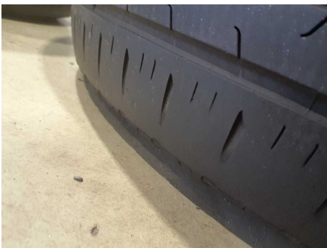
Damage 9: 2nd wheel set: 2 tyres - Does not meet the leasing specifications - Replace
