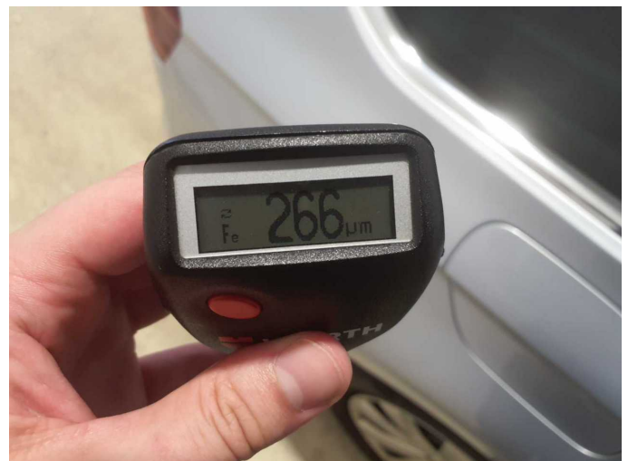
Repainting 2: Side panel - rear right side
