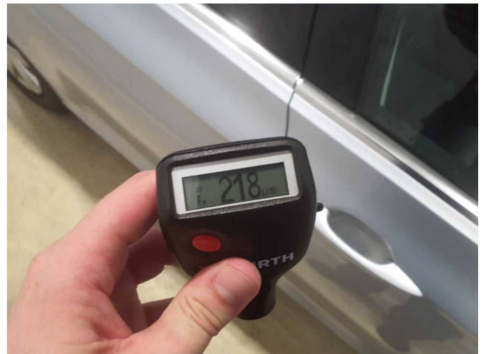
Repainting 1: Roof rail - right side
