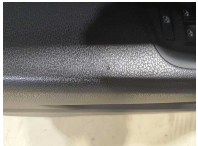
Damage 3: Trim / covers: Door trim - front left side - Burn hole (cigarettes) - Smart repair
