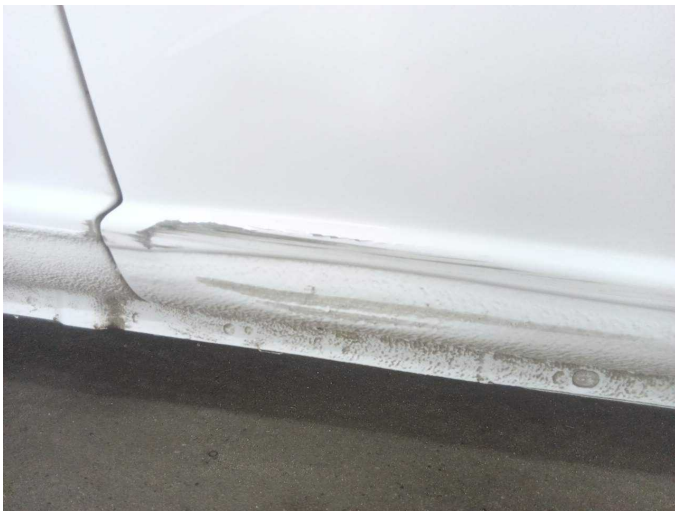
Damage 5: Sliding door, right: Sliding door - Damaged - Replace
