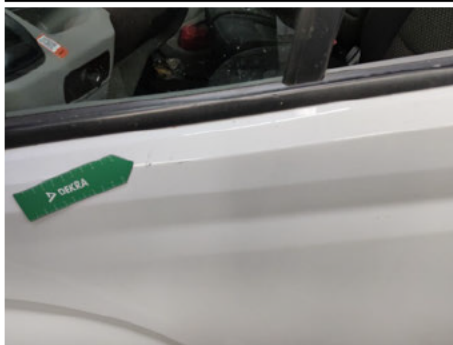
Tür / Vorne Links / Kratzer
