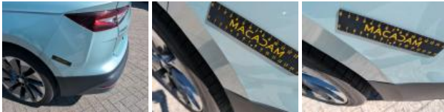
Bumper R, Dent(s) and scratch(es), Replace
