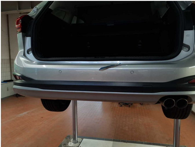
Damage 3: Rear bumper: Rear bumper - Scratched - Smart repair
