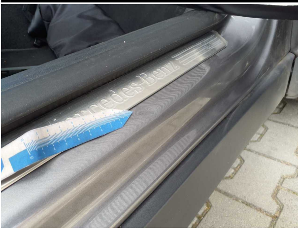
Damage #3: Sill - right side: Sill - Deformed - Smart repair
