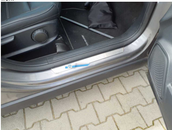
Damage #3: Sill - right side: Sill - Deformed - Smart repair
