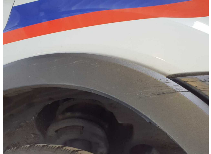
Damage 3: Mudguard - right side: Wheel well extension - Scratch(es) - Loss in value
