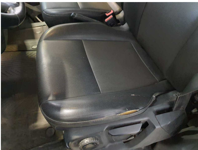
Damage 9: Seat - front: Seat cover - left side - Porous / cracked - Replace
