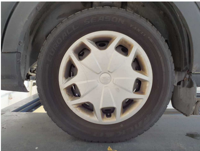
Damage 8: Wheel / tyres: Tyre - front - Worn - Replace
