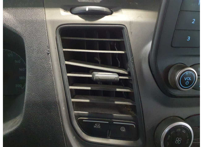
Damage 6: Instrument panel: Air nozzle - centre - Broken / torn - Replace
