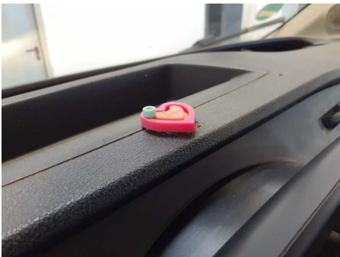
Damage 2: Instrument panel: Instrument panel (Mitte) - Glued / labelled - De-glue / neutralise
