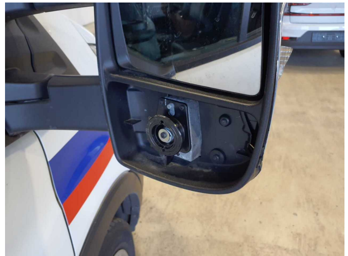
Damage 4: Wing mirror - right side: Mirror glass - Missing - Replace
