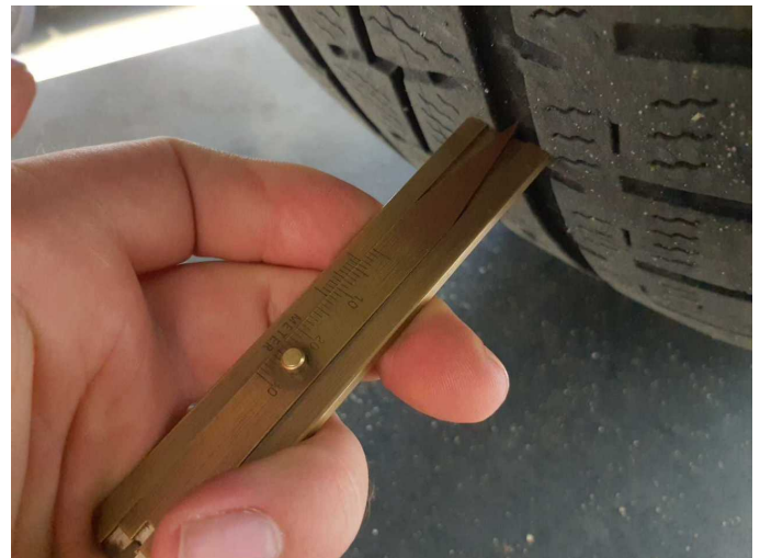
Damage 8: Wheel / tyres: Tyre - front - Worn - Replace
