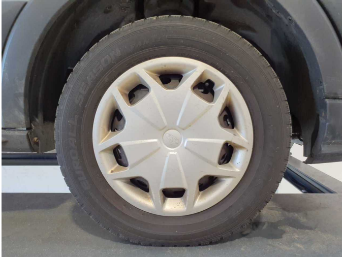
Damage 8: Wheel / tyres: Tyre - front - Worn - Replace
