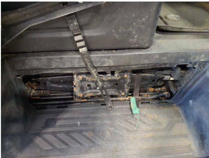
Damage 1: Trim / covers: Sill - front right side - Missing - Replace
