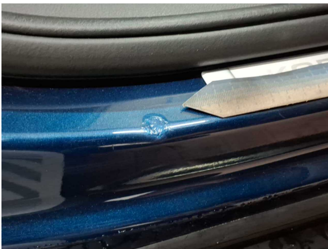
Damage 4: Sill - right side: Sill (5 AW) - Dent / paintcoat damage - Repair and paint
