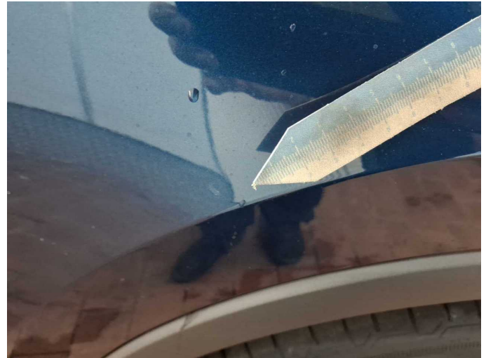
Damage 3: Mudguard - right side: Mudguard - right side - Dent / paintcoat damage - Smart repair
