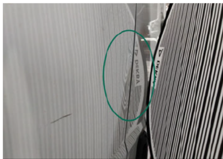
Heckklappe / Kofferraumtür / Mitte Links / Delle
