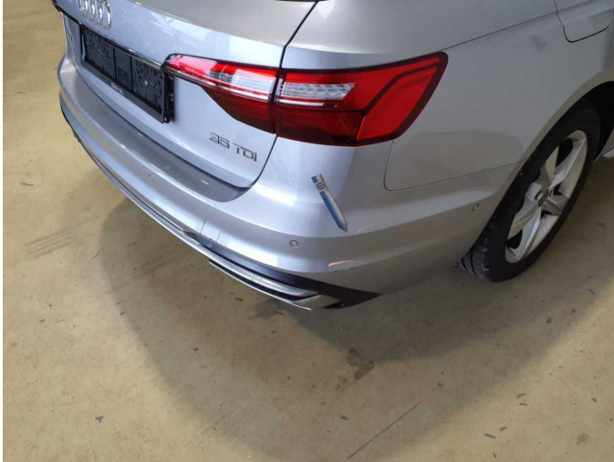
Damage 18: Rear bumper: Rear bumper (Inklusive anbauteile) - Dent / paintcoat damage - Replace
