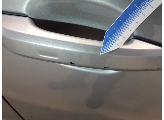
Damage 10: Door - front right side: Door handle - outside - Scratch(es) - Paint
