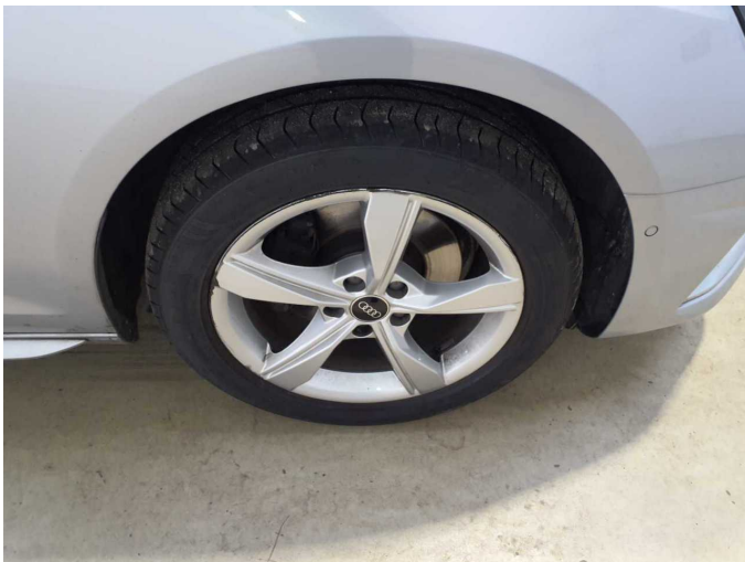
Damage 13: Wheel / tyres: Alloy rim - front right side - Scratch(es) - Replace
