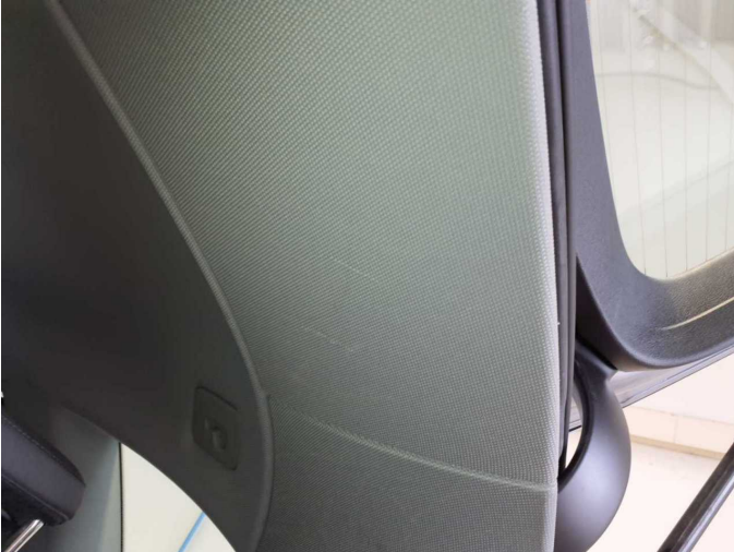
Damage 4: Trim / covers: Roof lining - Scratch(es) - Smart repair
