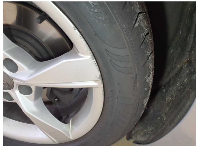
Damage 11: Wheel / tyres: Alloy rim - rear right side - Scratch(es) - Replace
