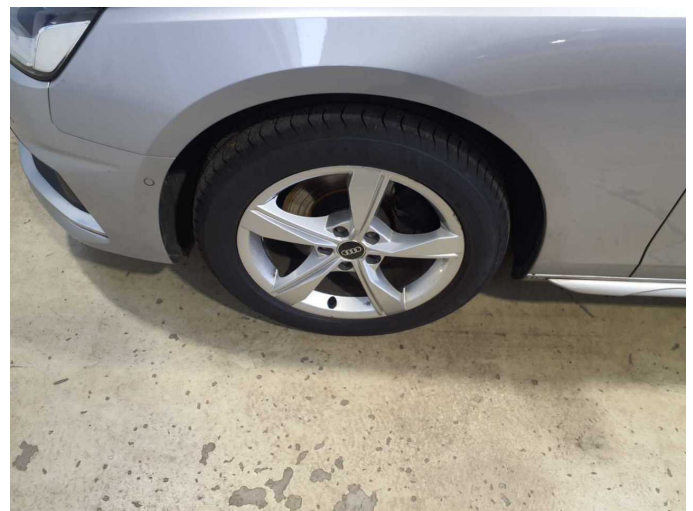
Damage 12: Wheel / tyres: Alloy rim - front left side - Scratch(es) - Replace
