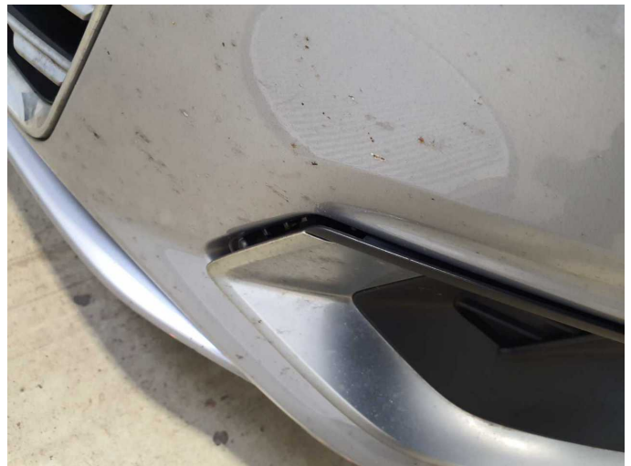
Damage 8: Trim / covers: Trim / covers - Broken / torn - Replace
