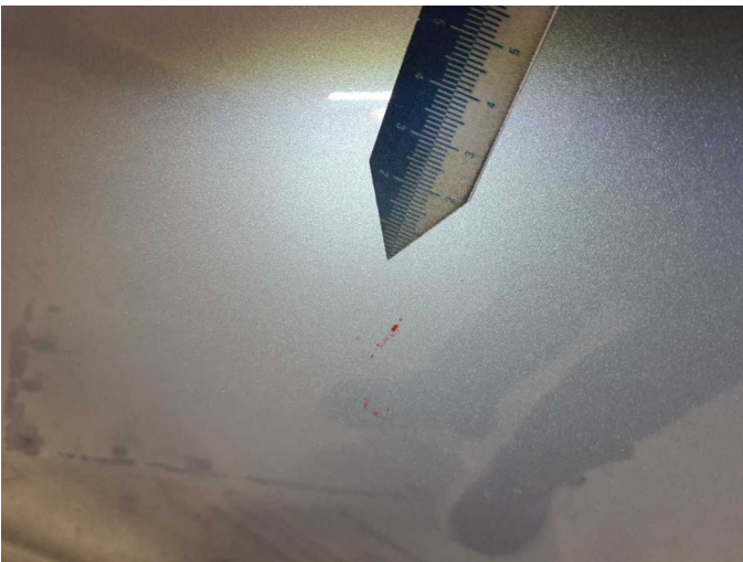
Damage 5: Door - front left side: Door - Scratch(es) - Smart repair
