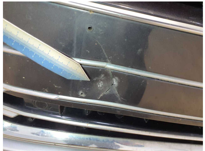
Damage 15: Front structure: Grille - Broken / torn - Replace
