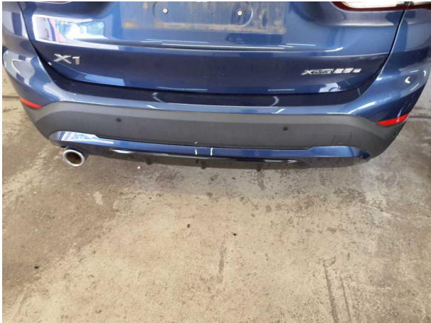
Damage #1: Rear bumper: Spoiler - Dent / paintcoat damage - Repair and paint
