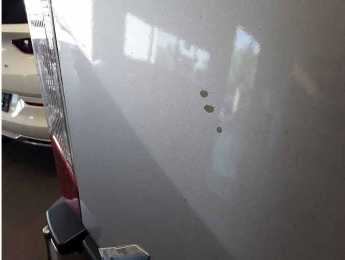
Damage 3: Boot lid / rear door: Rear door - left side - Paint defect - Smart repair
