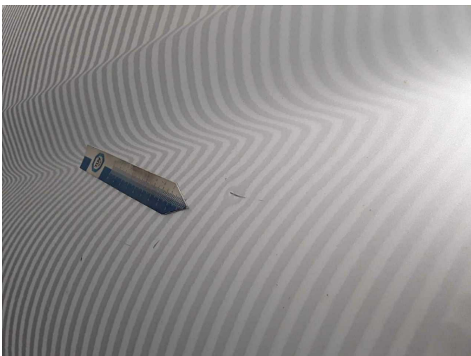
Damage 4: Door - rear right side: Door - Dent / paintcoat damage - Smart repair
