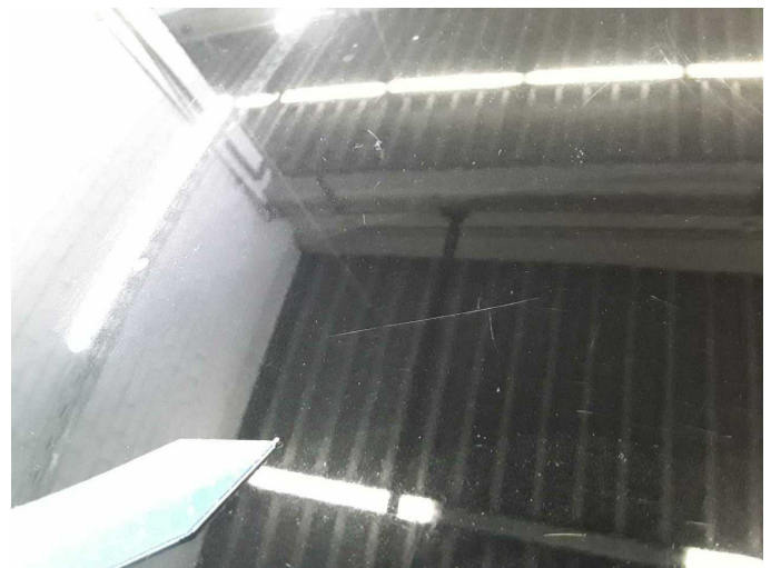
Damage 7: Bonnet: Bonnet - Scratch(es) - Paint
