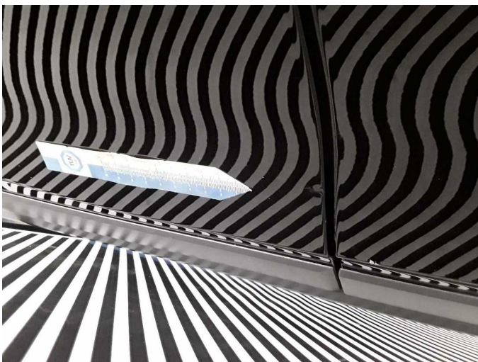
Damage 8: Door - rear right side: Door - Deformed - Repair and paint
