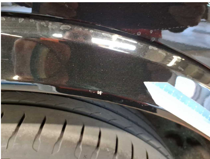
Damage 5: Side panel - rear left side: Wheel well extension - Scratched - Smart repair
