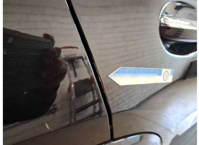
Damage 4: Door - rear right side: Door edge - Scratched - Smart repair
