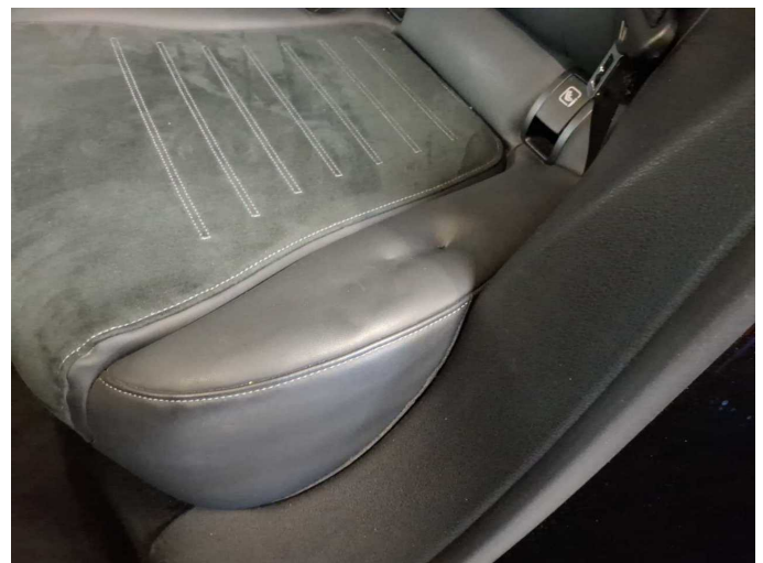
Damage 3: Seat - rear: Back seat - Deformed - Smart repair
