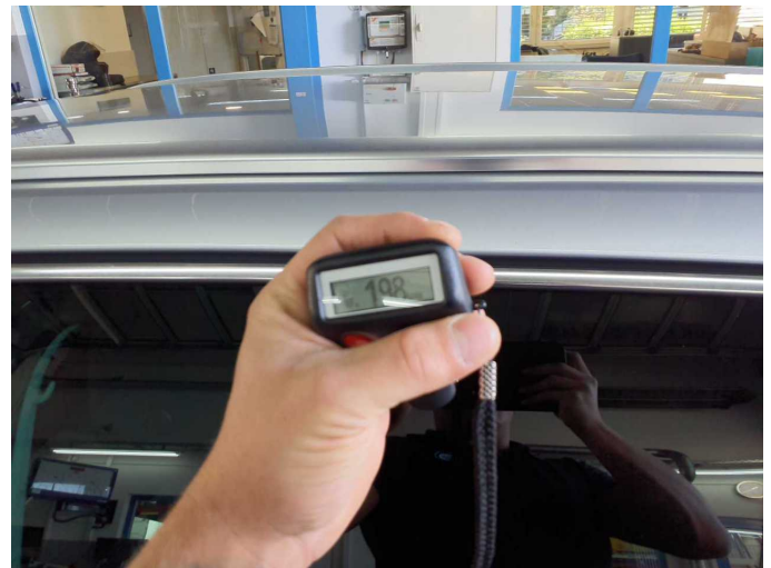
Roof rail - left side: 198 \mu\text{m}
