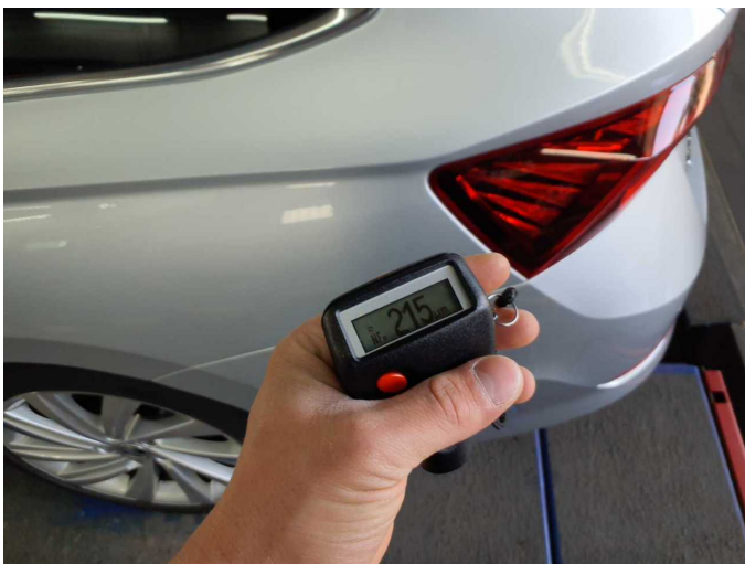
Side panel - rear left side: 215 \mu\text{m}
