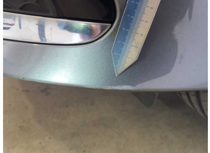
Damage 10: Front bumper: Front bumper - Scratch(es) - Paint
