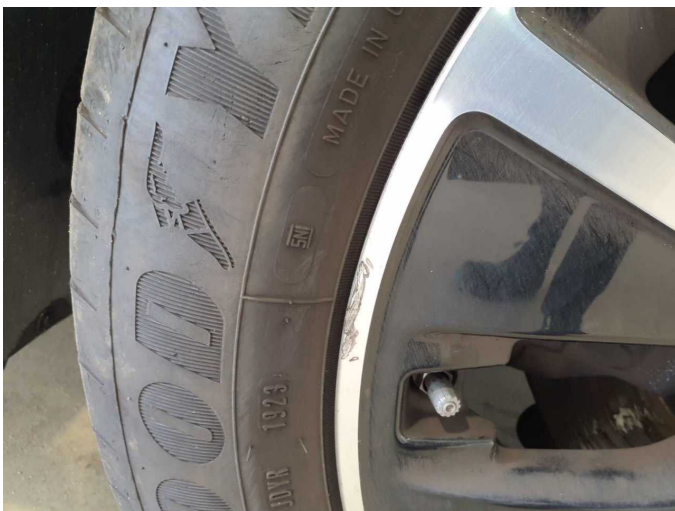
Damage 9: Wheel / tyres: Alloy rim - front right side - Scratch(es) - Replace
