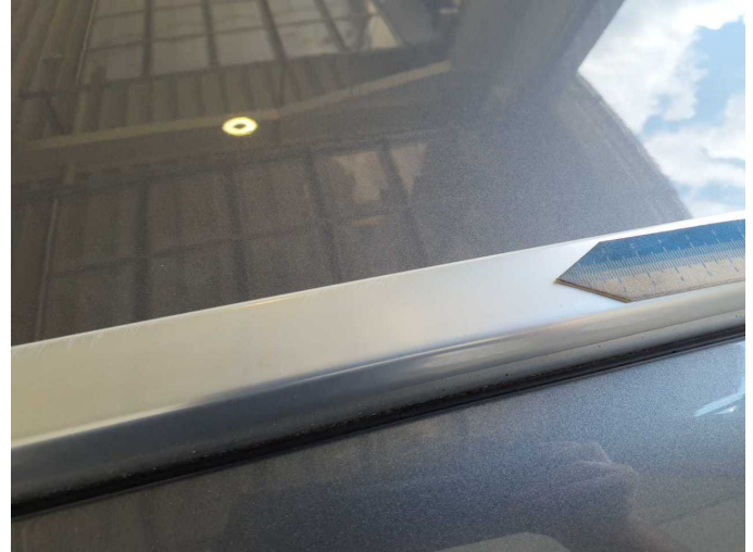
Damage 1: Roof: Roof rail - left side - Scratch(es) - Loss in value
