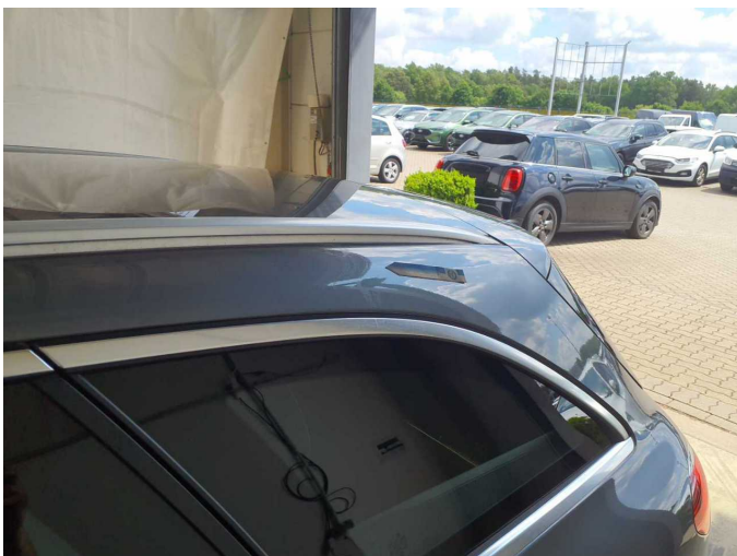
Damage 11: Roof: Roof rail - left side (Anätzung) - Paint defect - Repair and paint
