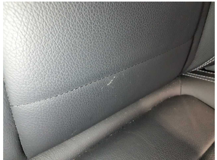
Damage 5: Seat - front: Seat cover - right side - Scratch(es) - Smart repair
