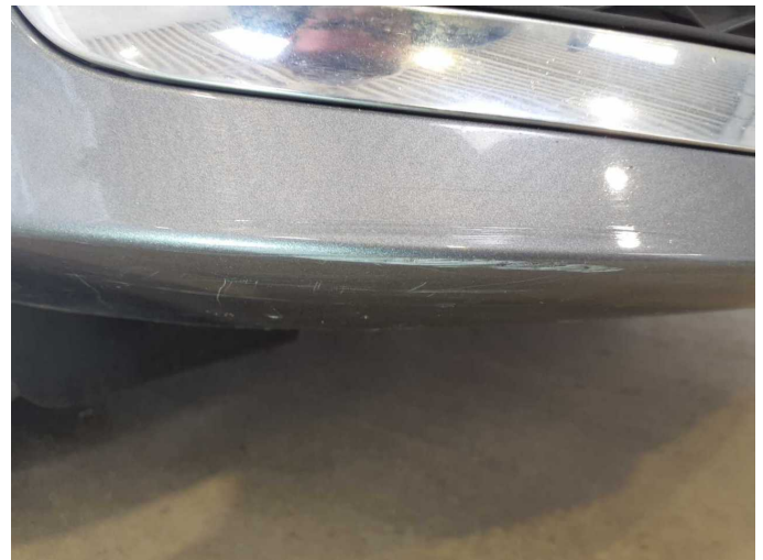
Damage 10: Front bumper: Front bumper - Scratch(es) - Paint
