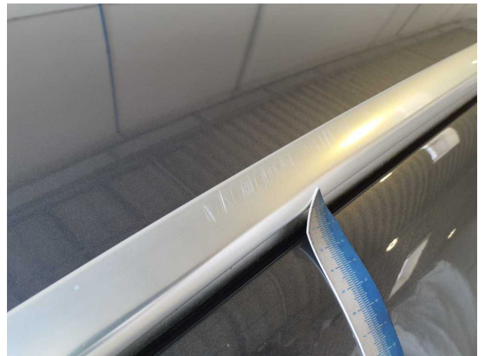
Damage 2: Roof: Roof rail - right side - Scratch(es) - Loss in value
