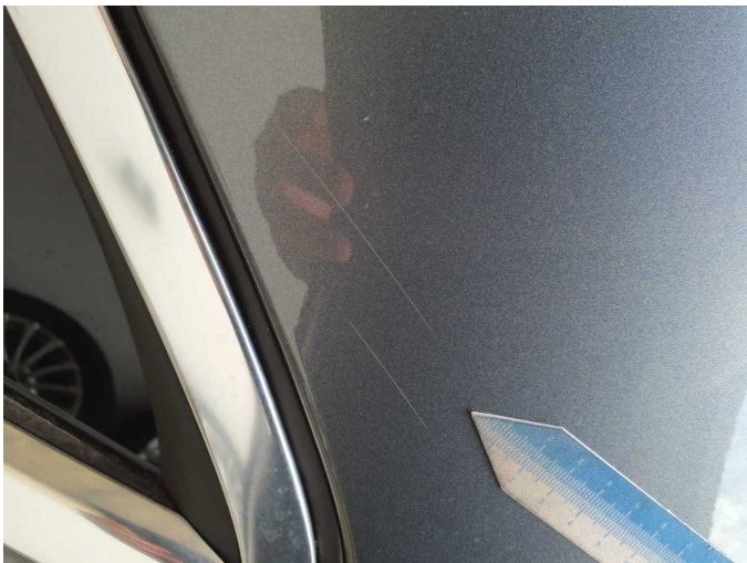
Damage 12: Side panel - rear left side: Side panel - Dent / paintcoat damage - Repair and paint
