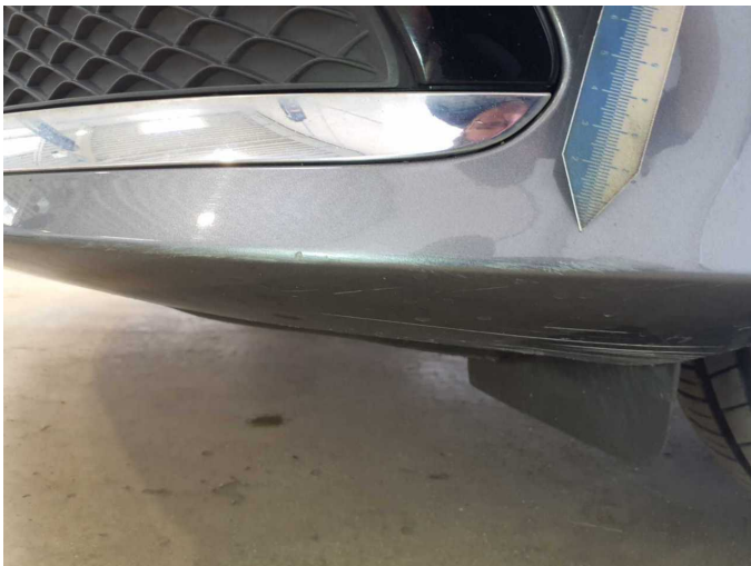
Damage 10: Front bumper: Front bumper - Scratch(es) - Paint
