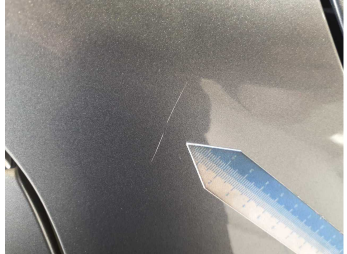
Damage 7: Mudguard - right side: Mudguard - right side - Scratch(es) - Smart repair
