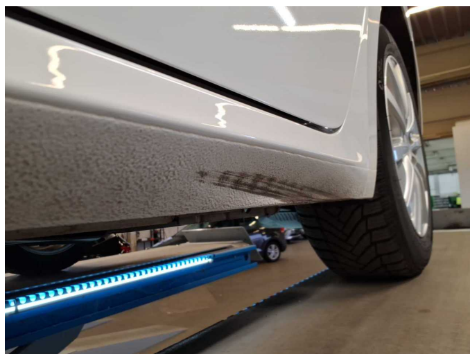
Damage 5: Sill - left side: Sill - Damaged - Paint
