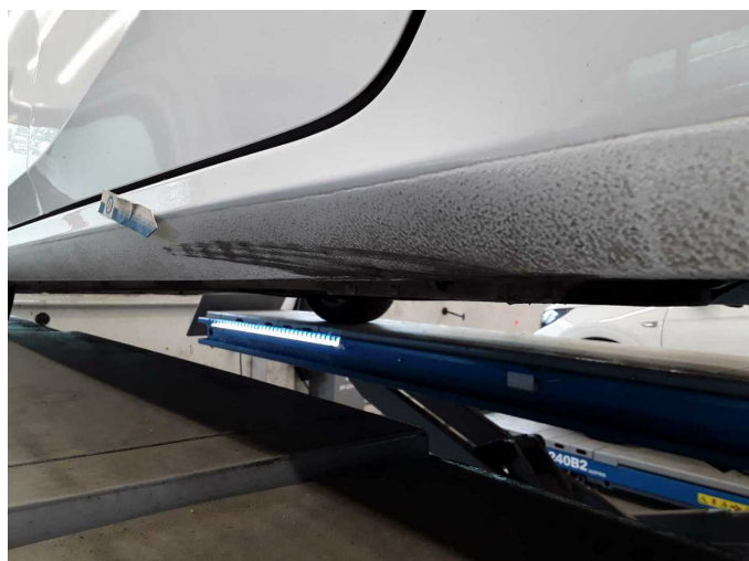
Damage 5: Sill - left side: Sill - Damaged - Paint
