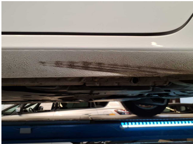
Damage 5: Sill - left side: Sill - Damaged - Paint
