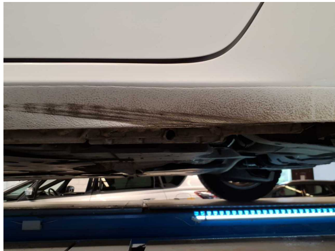
Damage 5: Sill - left side: Sill - Damaged - Paint
