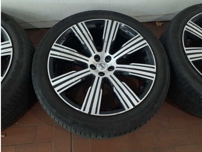
Damage 8: 2nd wheel set: 1 alloy rim - Scratch(es) - Replace
