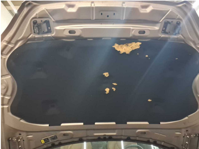
Damage 4: Bonnet: Insulation lining - Holes - Replace
