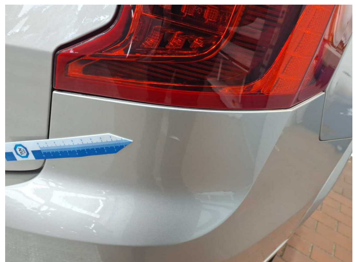
Damage 5: Rear bumper: Rear bumper - Scratch(es) - Paint
