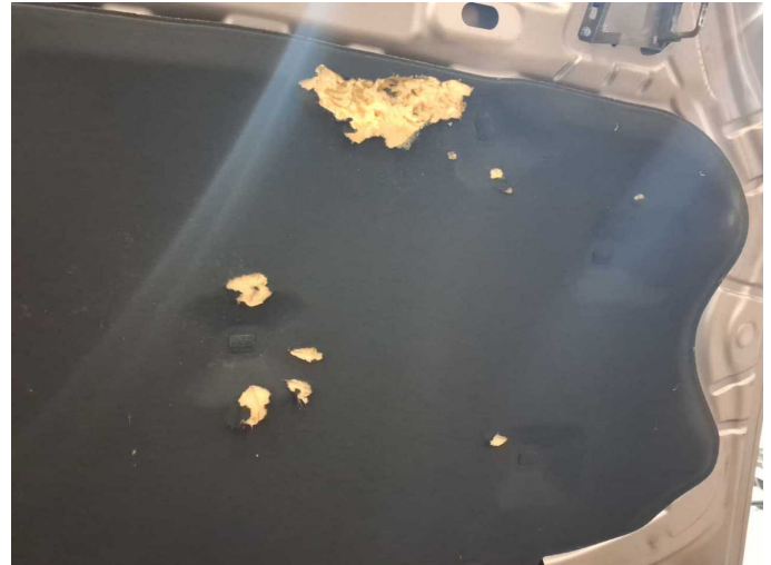
Damage 4: Bonnet: Insulation lining - Holes - Replace
