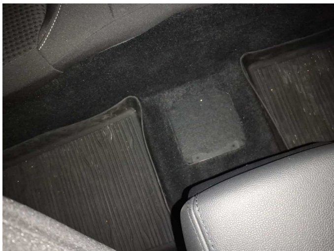
Damage 7: Trim / covers: Carpet - Damaged - Replace
