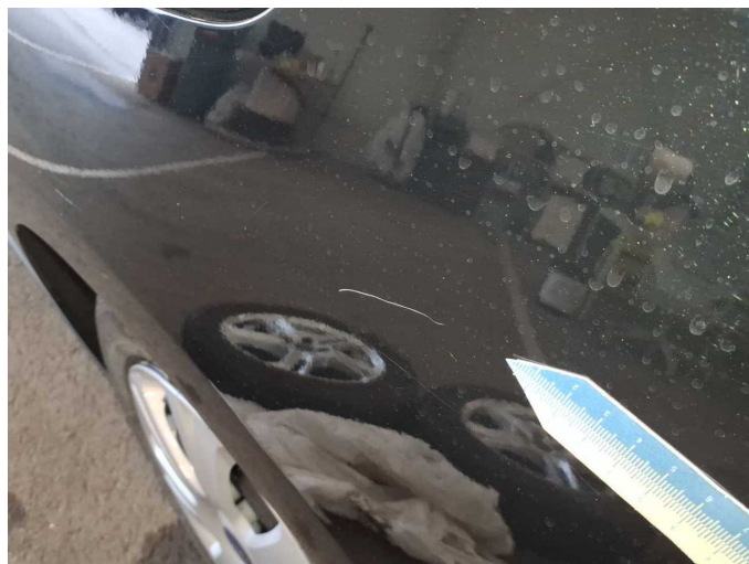
Damage 8: Side panel - rear left side: Side panel - Scratch(es) - Paint
