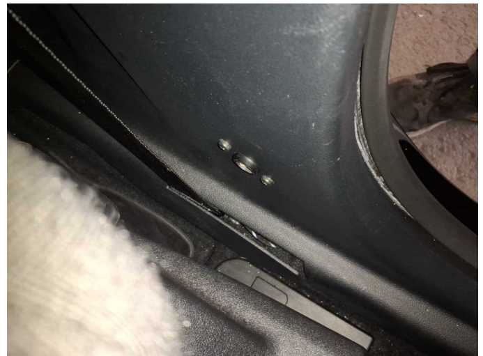
Damage 4: Trim / covers: B-pillar - trim - interior, left side - Damaged - Replace
