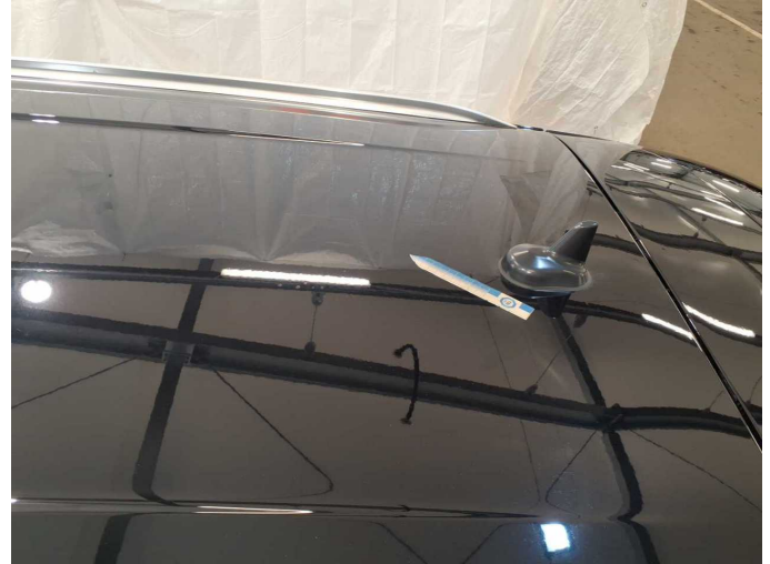
Damage 3: Roof: Roof - dent(s) - Smooth repair work
