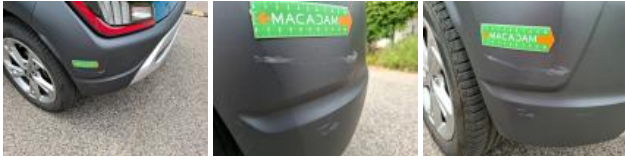
Bumper moulding R, Scratch(es), Replace
