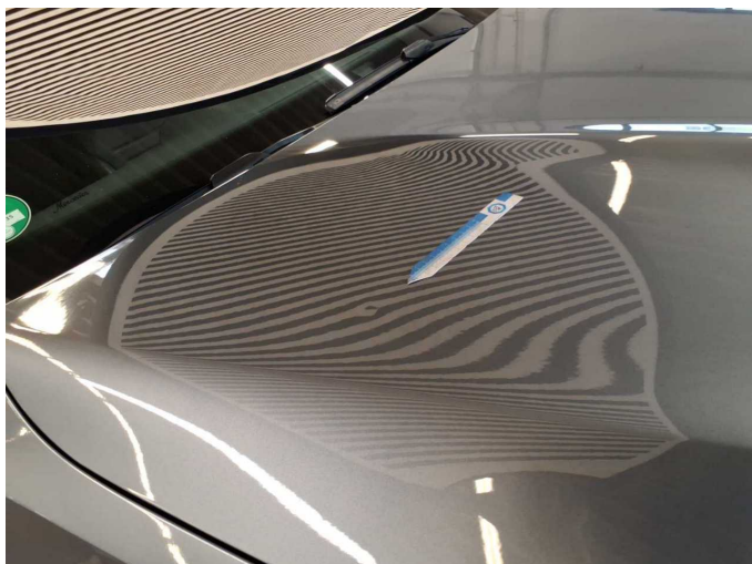
Damage 1: Bonnet: Bonnet - dent(s) - Smooth repair work
