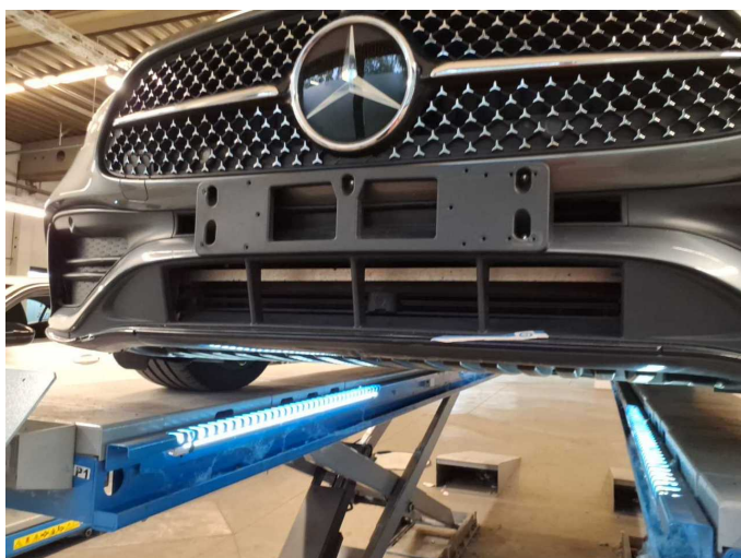
Damage 11: Front bumper: Front bumper (Materialabtrag) - Scratched - repair according to calculation
