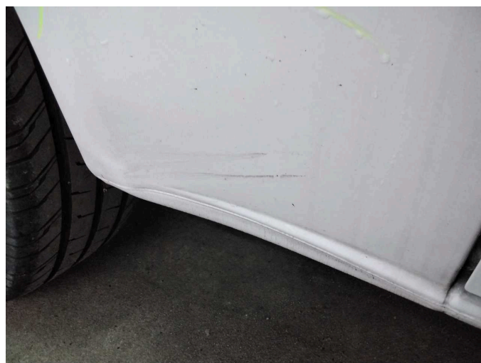
Damage 3: Side panel - rear right side: Side panel - Dent / paintcoat damage - Repair and paint
