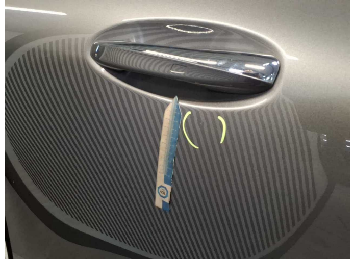
Wear and tear 2: Door - rear left side: Door - dent(s) - Smooth repair work
