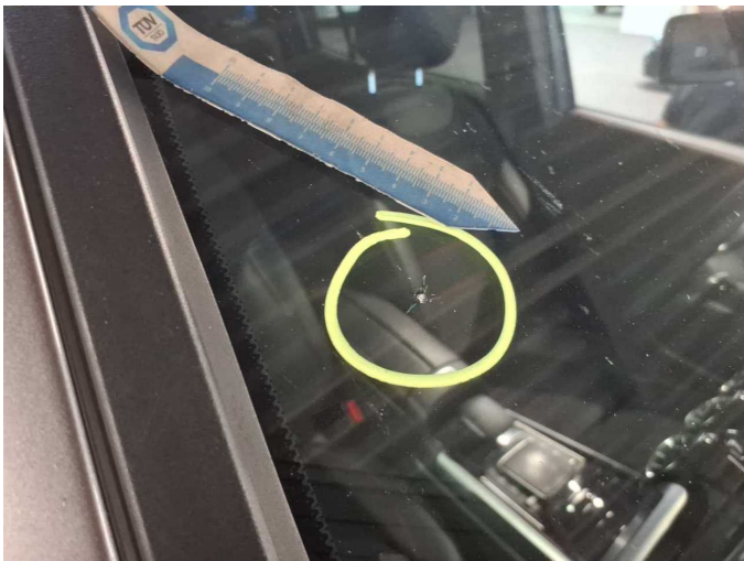
Damage 14: Vehicle glazing: Windscreen - Stone chips - repair according to calculation
