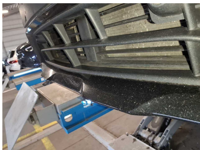
Damage 7: Front bumper: Spoiler (Sandstrahleffekt) - Stone chips - Paint
