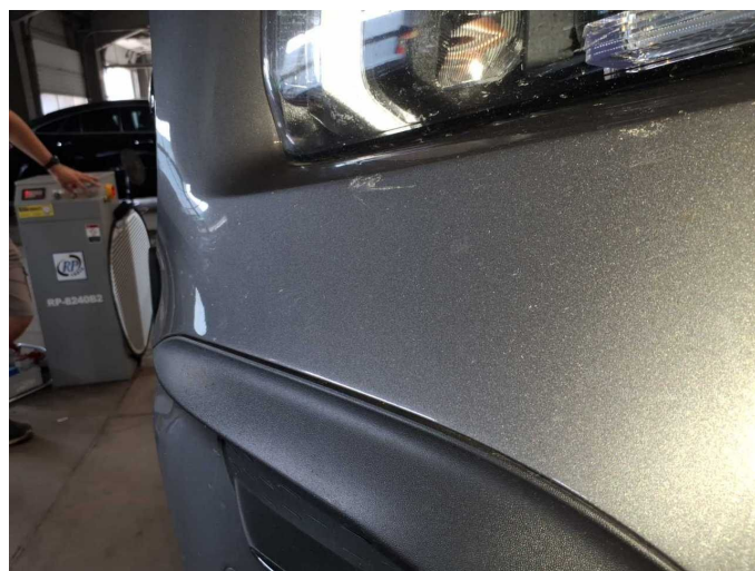
Damage 13: Front bumper: Front bumper (Sandstrahleffekt) - Stone chips - Paint
