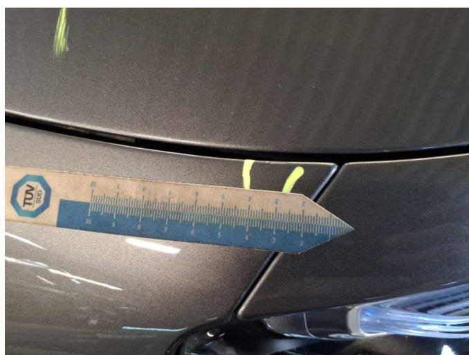
Damage 6: Mudguard - right side: Mudguard - right side - Scratched - Smart repair
