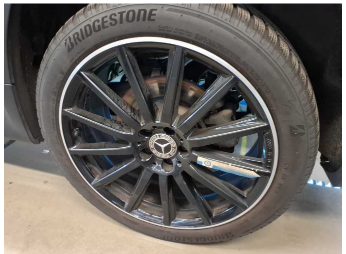
Wear and tear 1: Wheel / tyres: Alloy rim - rear left side - Scratch(es) - No deduction
