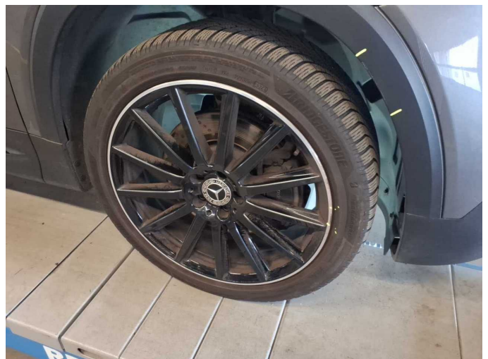
Damage 10: Wheel / tyres: Alloy rim - front right side - Scratched - Loss in value
