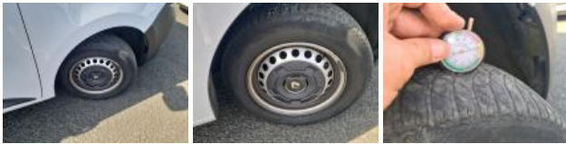
Tyre FL, Out of tolerance, Replace
