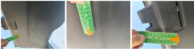
Boot lid covering R, Scratch(es), Replace
