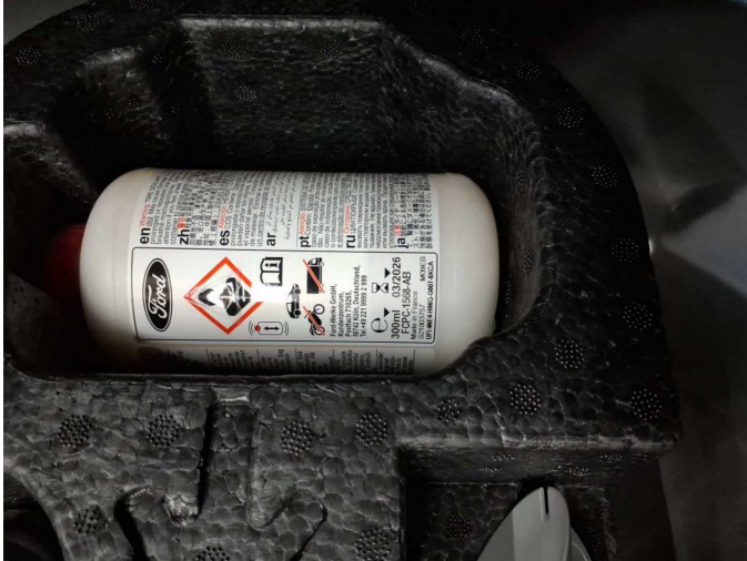
Damage 2: Equipment: Tirefit filler - Expired - Replace
