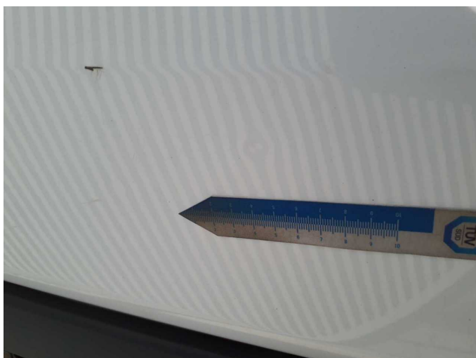
Damage 4: Boot lid / rear door: Rear door - left side - Dent / paintcoat damage - Smart repair
