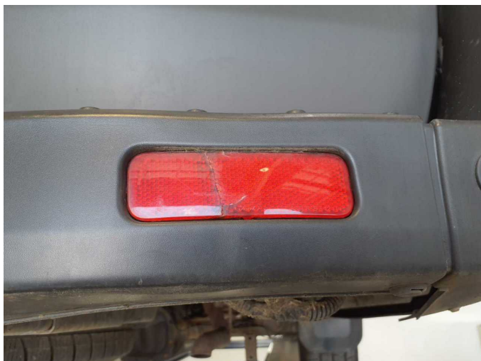
Damage 1: Rear bumper: Reflector - right side - Broken / torn - Replace
