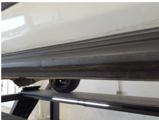
Damage 7: Sill - right side: Trim - Scratch(es) - Replace
