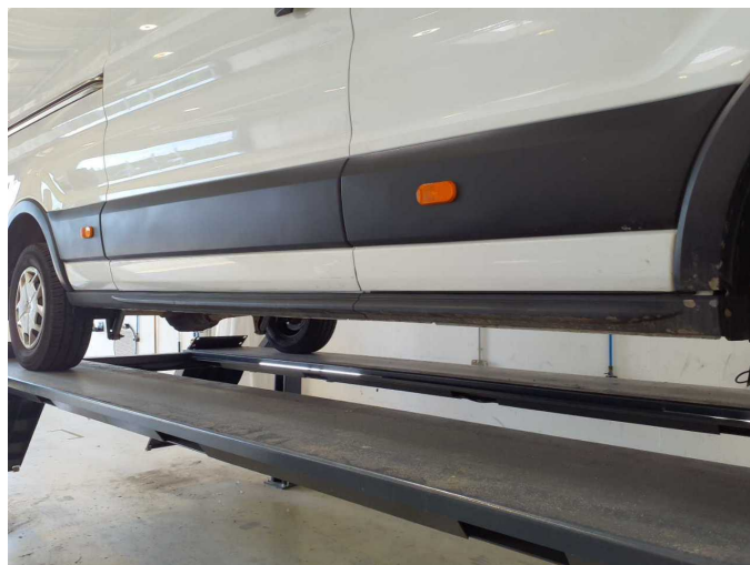
Damage 7: Sill - right side: Trim - Scratch(es) - Replace
