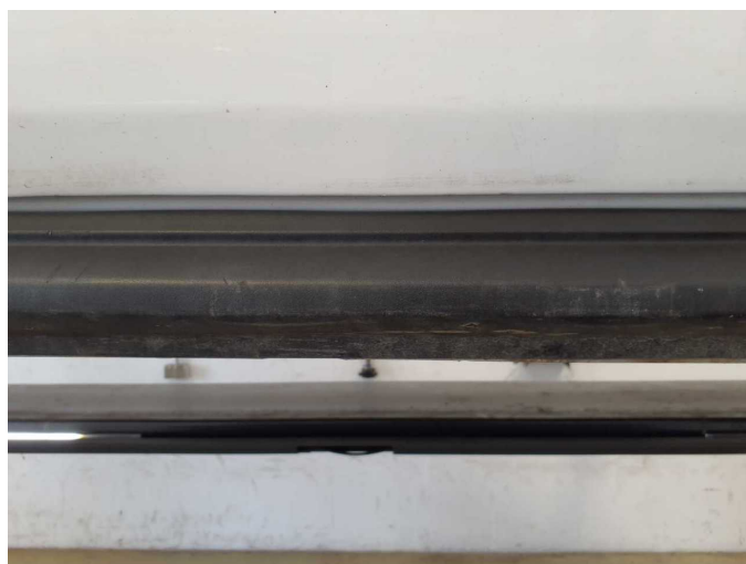
Damage 7: Sill - right side: Trim - Scratch(es) - Replace
