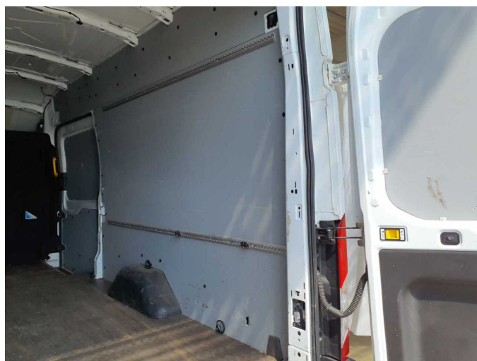
Damage 6: Trim / covers: Cargo area - lining - right side - Holes - Replace
