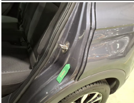
Door sill / Back Left / Scratched
