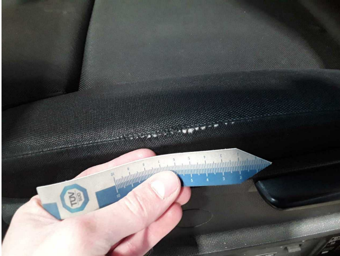
Damage 3: Seat - front: Seat cover - left side - Broken / torn - Replace
