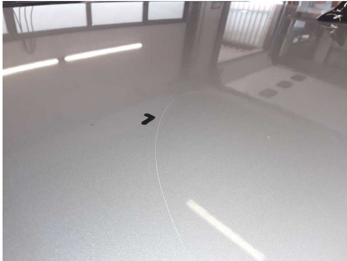
Damage 16: Roof: Roof - Scratch(es) - Paint
