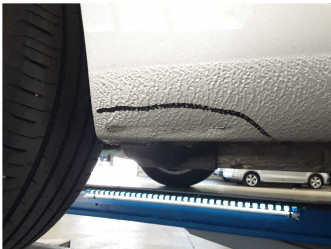
Damage 10: Sill - right side: Sill - Scratched - Repair and paint
