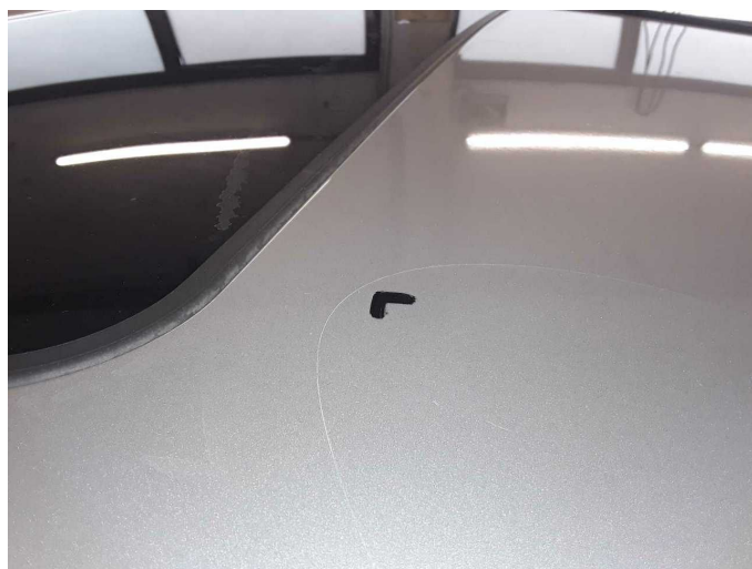
Damage 16: Roof: Roof - Scratch(es) - Paint
