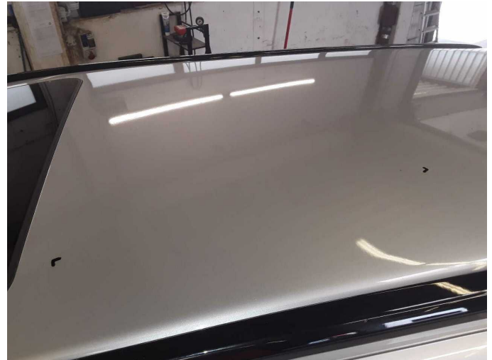
Damage 16: Roof: Roof - Scratch(es) - Paint
