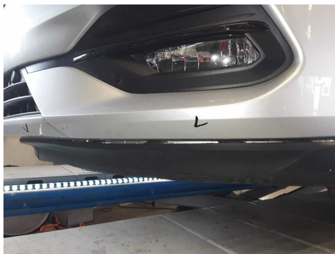
Damage 12: Front bumper: Front bumper - Scratched - Paint
