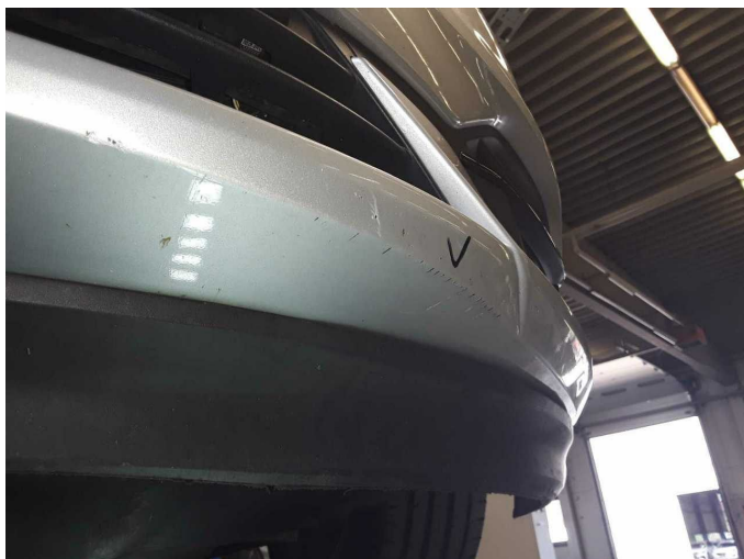
Damage 12: Front bumper: Front bumper - Scratched - Paint
