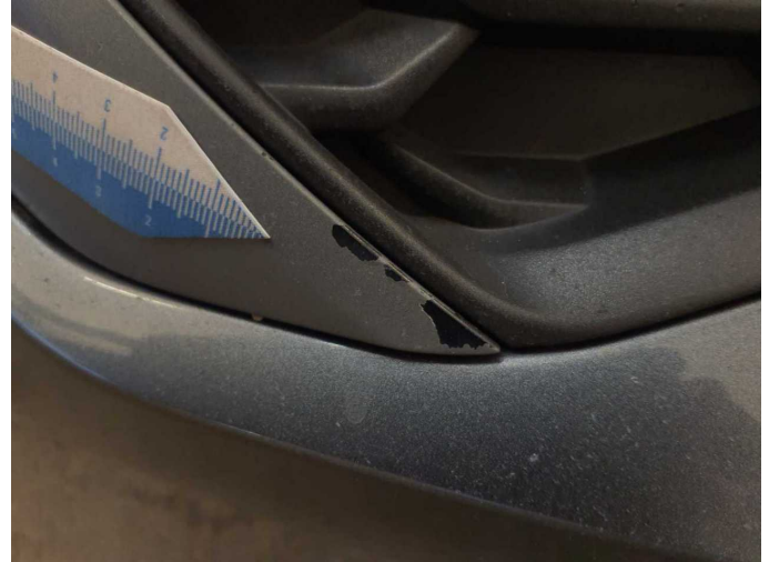
Damage 4: Trim / covers: Brightware / decorative strip - Paint defect - Smart repair
