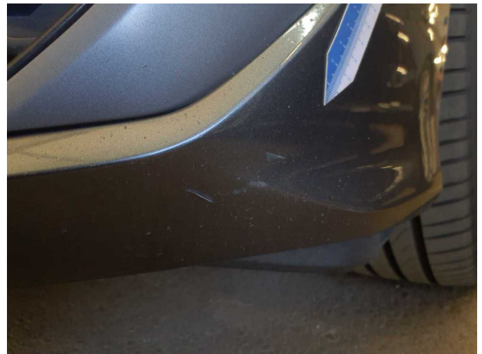
Damage 5: Front bumper: Front bumper - Scratch(es) - Paint
