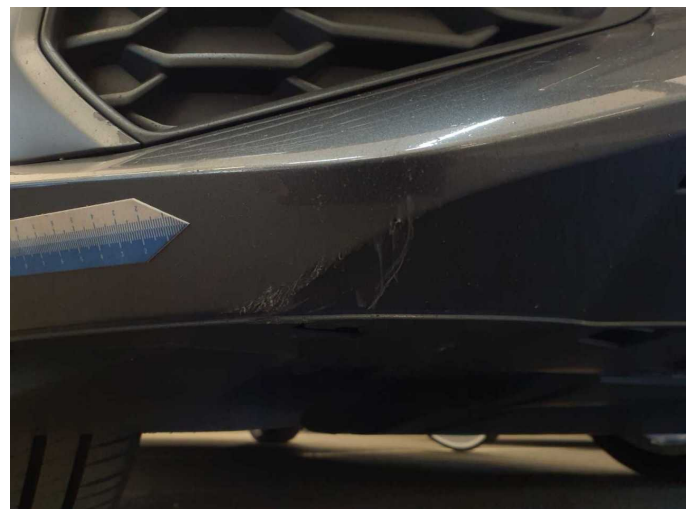
Damage 5: Front bumper: Front bumper - Scratch(es) - Paint
