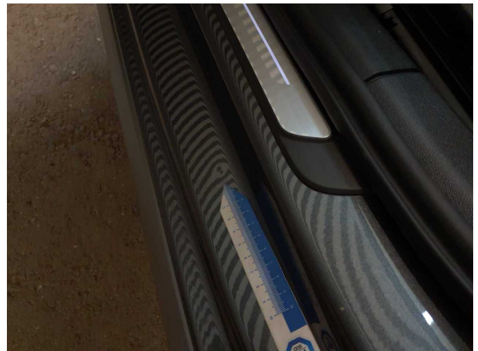
Damage 2: Sill - left side: Sill - dent(s) - Smart repair
