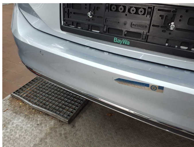
Damage 5: Rear bumper: Rear bumper - Scratch(es) - Paint
