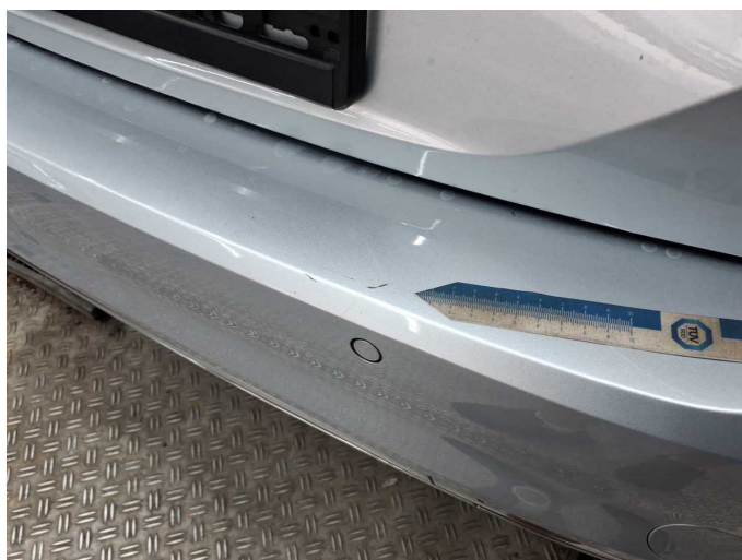
Damage 5: Rear bumper: Rear bumper - Scratch(es) - Paint
