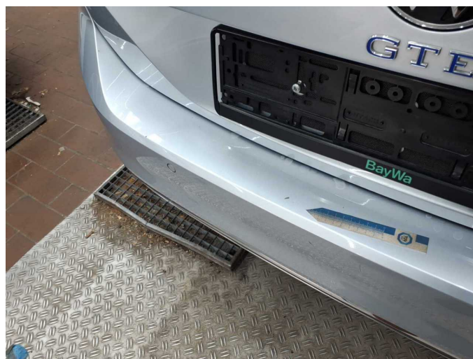
Damage 5: Rear bumper: Rear bumper - Scratch(es) - Paint
