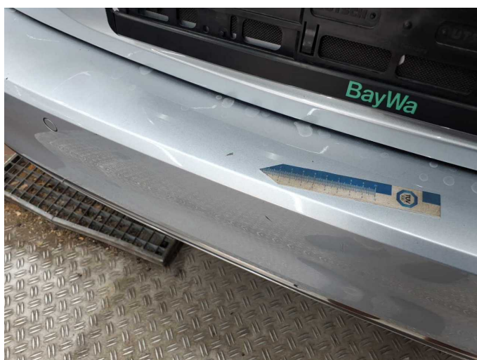
Damage 5: Rear bumper: Rear bumper - Scratch(es) - Paint
