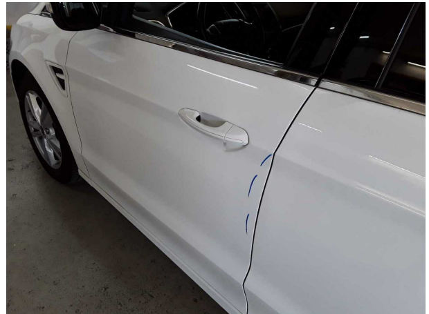
Beschädigung #5: Tür vorn links: Tür - Lackmangel - Smart Repair
