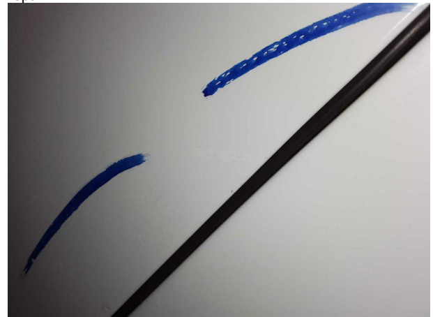
Damage #5: Door - front left side: Door - Paint defect - Smart repair
