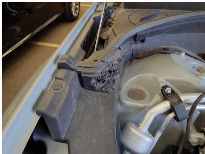
Damage 1: Engine: Engine cover (Dichtung L + R) - Damage caused by marten / rodent - Replace
