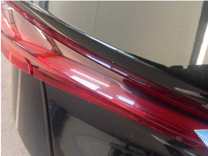
Damage 2: Tail light: Auxiliary brake light (Bremsleuchte/Lichtband Heckklappe) - Broken / torn - Replace
