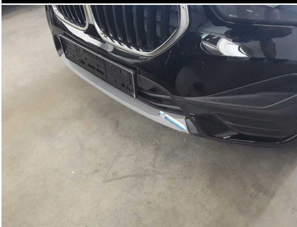
Damage #4: Front bumper: Air-inlet grille (Blende mitte unten) - Deformed - Replace
