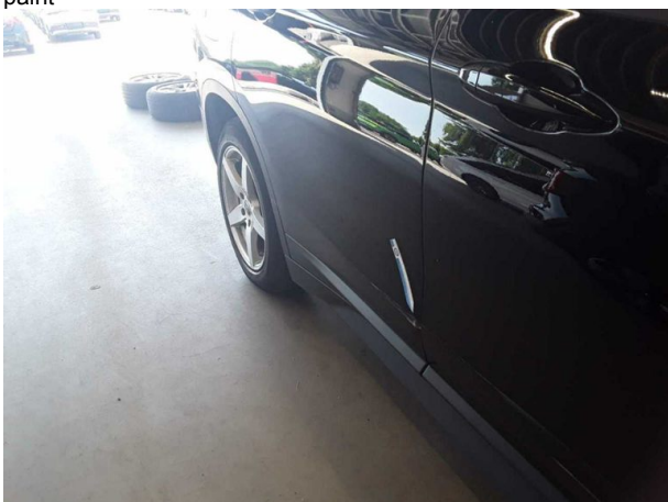
Damage #11: Door - rear right side: Door - Deformed - Replace
