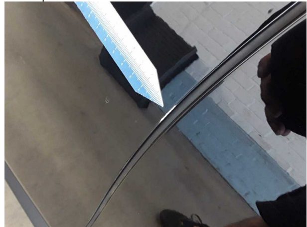
Damage #2: Door - front left side: Door edge - Scratched - Cover / polish
