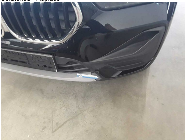
Damage #6: Front bumper: Front bumper (unpainted) - Scratched - Replace
