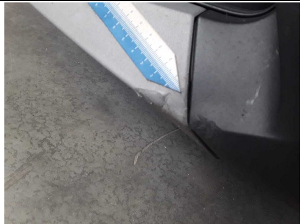
Damage #4: Front bumper: Air-inlet grille (Blende mitte unten) - Deformed - Replace
