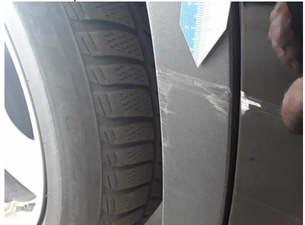
Damage #5: Side panel - rear right side: Wheel well extension... - Scratched - Replace
