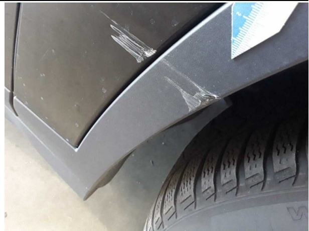
Damage #7: Mudguard - right side: Wheel well extension - Scratched - Replace
