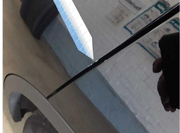
Damage #1: Door - rear left side: Door edge - Scratched - Cover / polish
