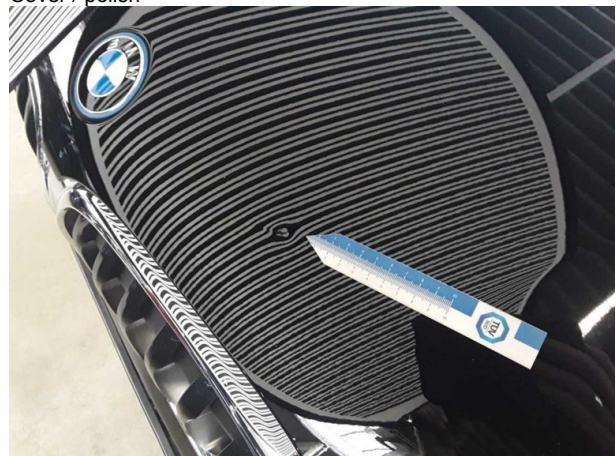
Damage #3: Bonnet: Bonnet - dent(s) - Smooth repair work
