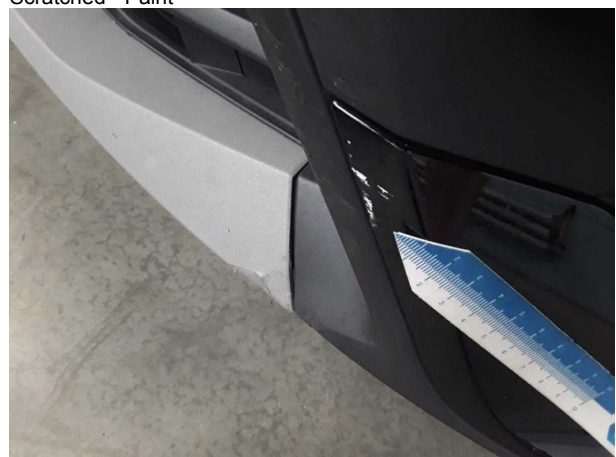
Damage #9: Front bumper: Front bumper - Scratched - Repair and paint
