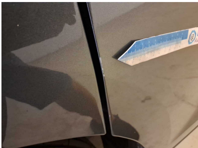
Damage 4: Sliding door, right: Sliding door with glass panel (Türkante) - Scratch(es) - Smart repair
