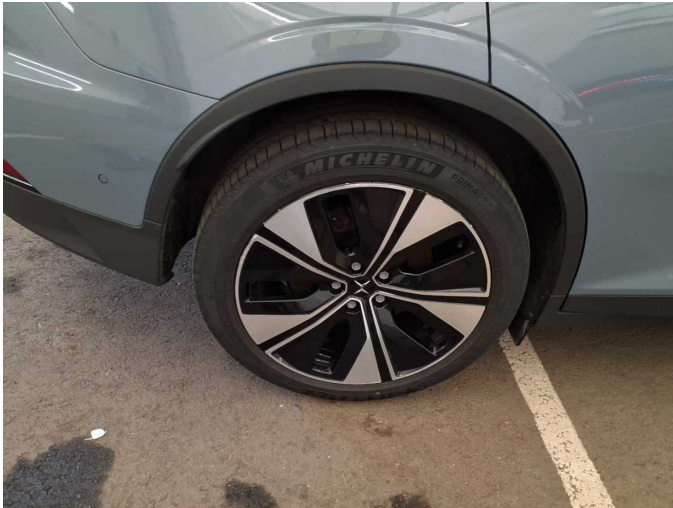
Damage 3: Wheel / tyres: Alloy rim - rear right side (Materialabtrag) - Scratched - Replace
