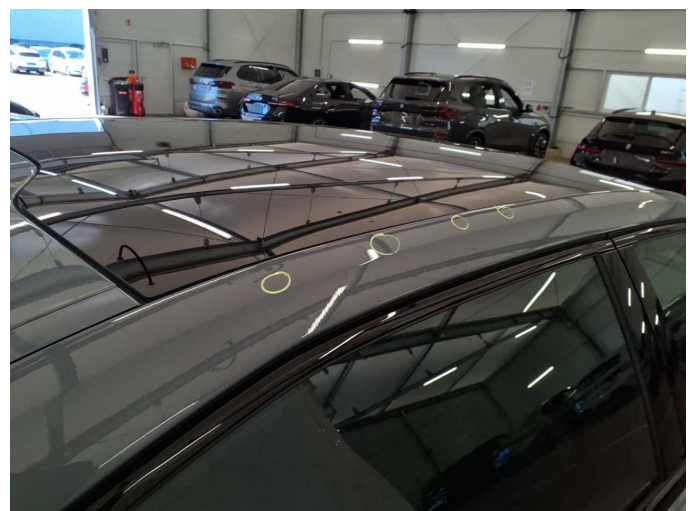
Damage 4: Body: Body - Damage by hail - repair according to calculation
