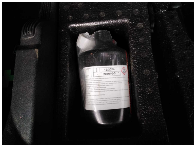
Damage 1: Equipment: Tirefit filler - Expired - Replace
