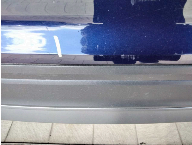
Damage 12: Rear bumper: Rear bumper - Scratch(es) - Paint
