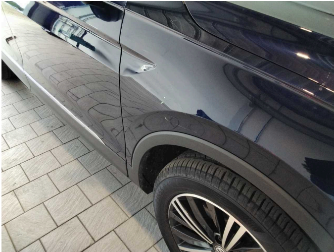
Damage 15: Mudguard - right side: Mudguard - right side - Scratch(es) - Paint
