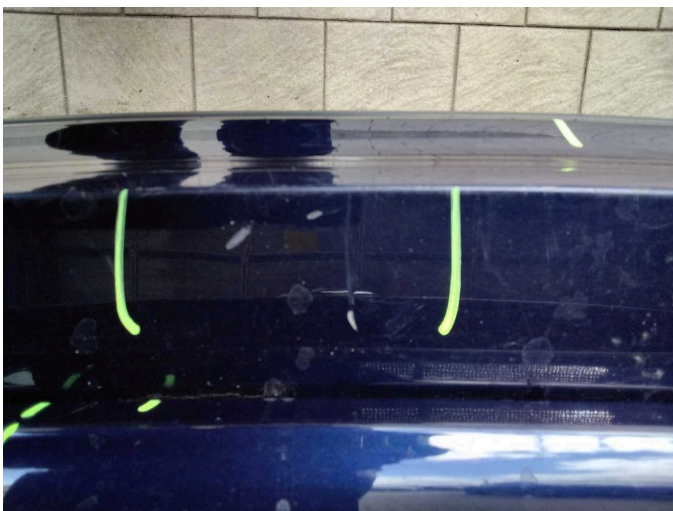
Damage 12: Rear bumper: Rear bumper - Scratch(es) - Paint
