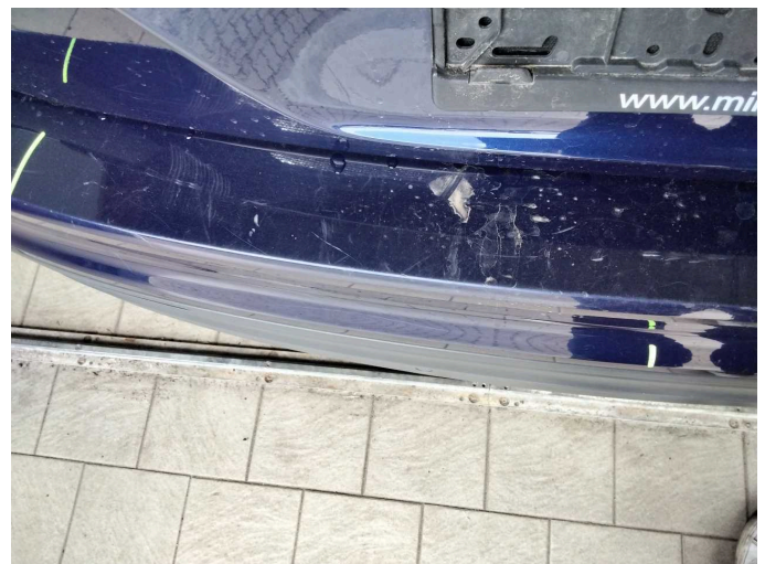
Damage 12: Rear bumper: Rear bumper - Scratch(es) - Paint
