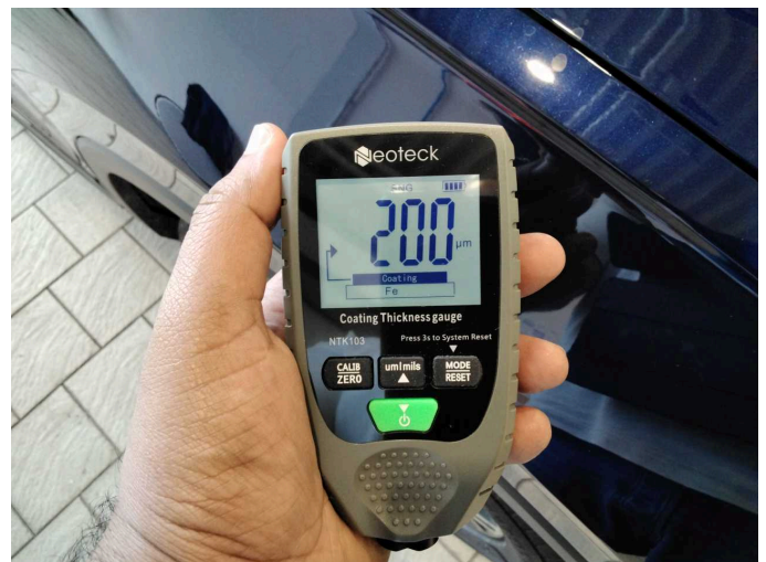
Mudguard - right side: 200 µm
