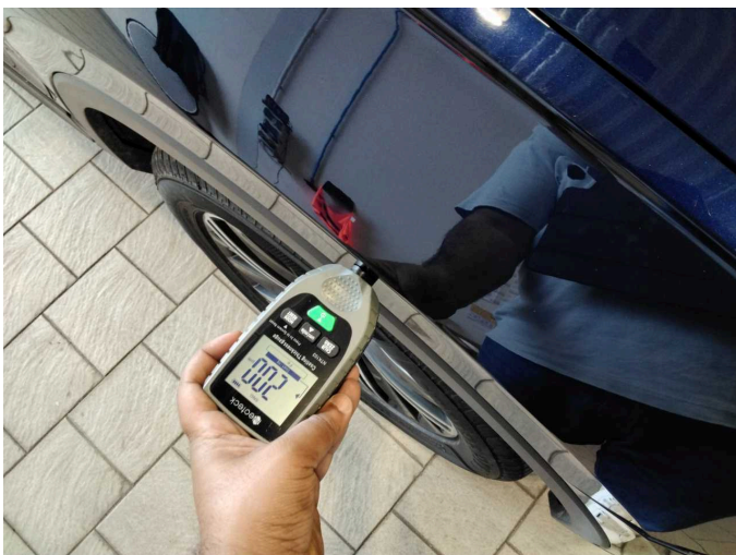
Mudguard - right side: 200 µm
