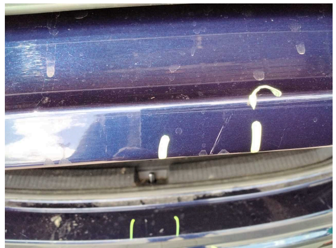
Damage 14: Boot lid / rear door: Boot lid - Dent / paintcoat damage - Repair and paint
