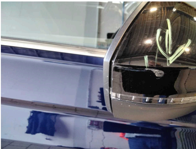
Damage 11: Wing mirror - right side: Cap - Scratch(es) - Replace
