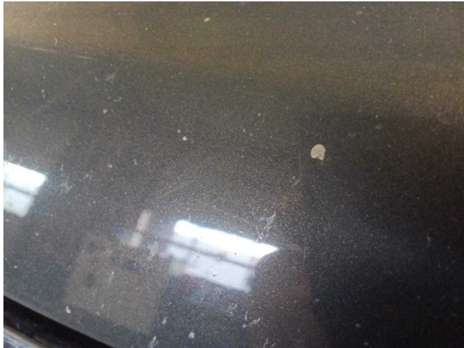
Damage 13: Bonnet: Bonnet - Stone chips - Paint
