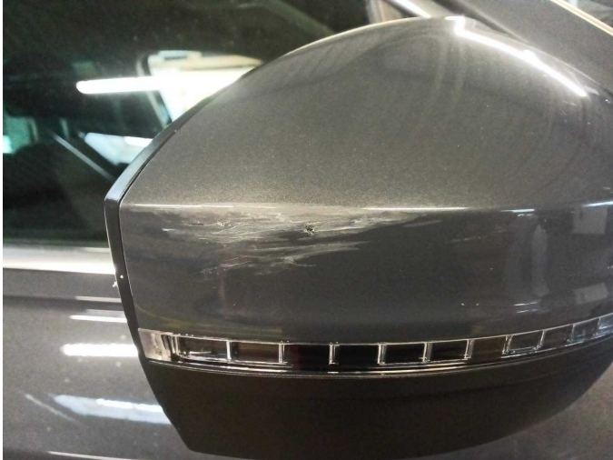
Damage 10: Wing mirror - right side: Mirror housing - Scratch(es) - Paint
