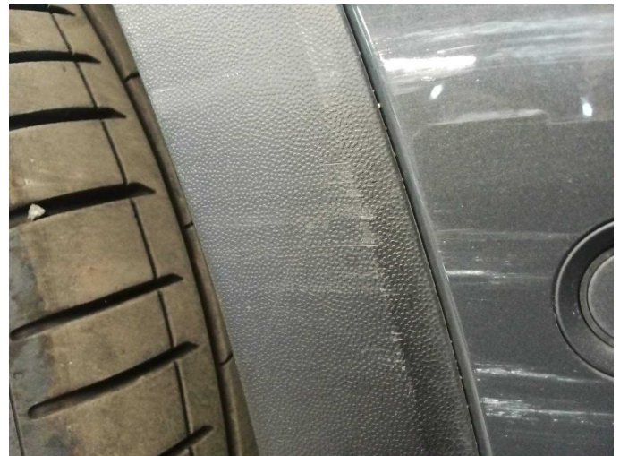
Damage 11: Mudguard - right side: Wheel well extension - Scratched - Replace
