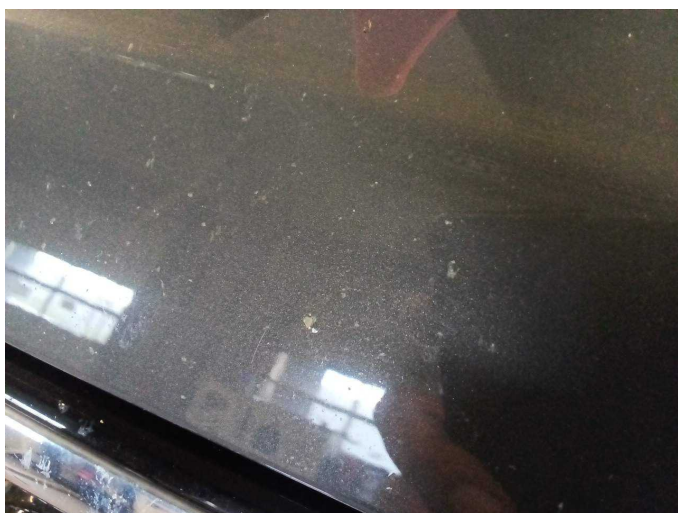
Damage 13: Bonnet: Bonnet - Stone chips - Paint
