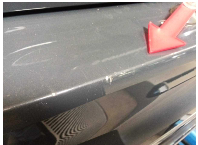
Damage 12: Rear bumper: Rear bumper - Scratch(es) - Paint
