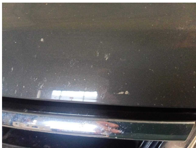
Damage 13: Bonnet: Bonnet - Stone chips - Paint
