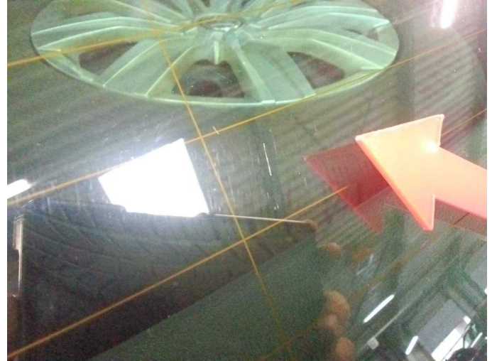
Damage 15: Vehicle glazing: Rear window - Scratch(es) - Replace
