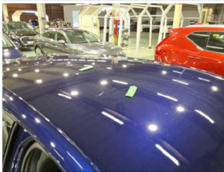
Roof / Exterior Exterior / Paint etching
