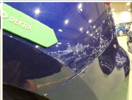
Wing / Back Left / Improper Repair
