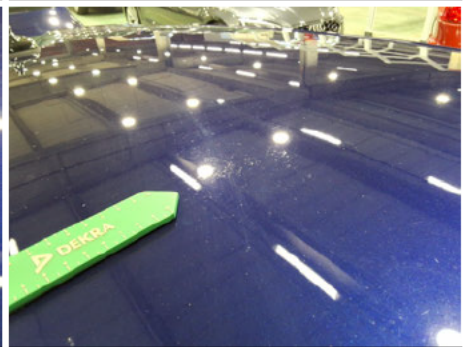
Roof / Exterior Exterior / Paint etching
