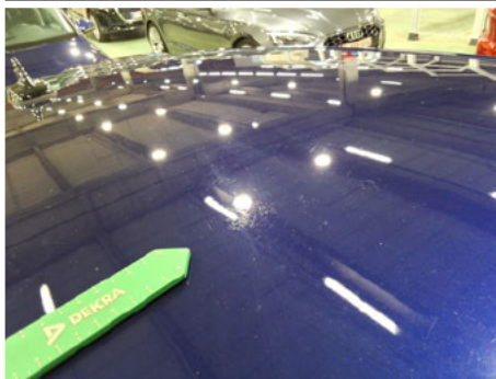
Roof / Exterior Exterior / Paint etching
