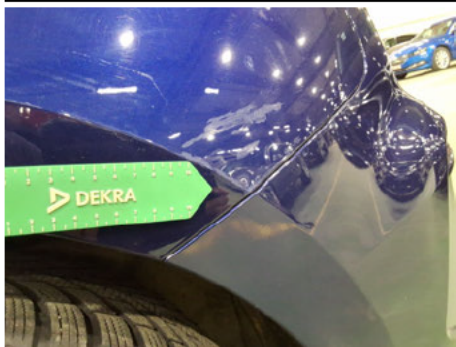
Wing / Back Left / Improper Repair
